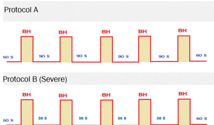
Figure 6-3 Two Breath Hold (BH) Protocols Simulating Sleep Apnea (Protocol B is More Severe Form of Sleep Apnea Compared to Protocol A) (Alex R. M., 2010)
