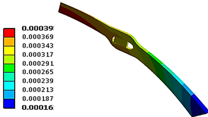
Figure 4-15: Representative FE model displacement results in meters of cornea segment with 5 mm diameter Myring with (0.5 \times 0.3) \text{ mm}^2 cross section
