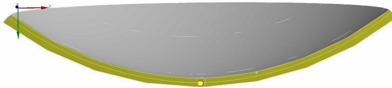
Figure 6-5: Modeling of the symmetrical plane BC fixed in horizontal plane and free in vertical plane
