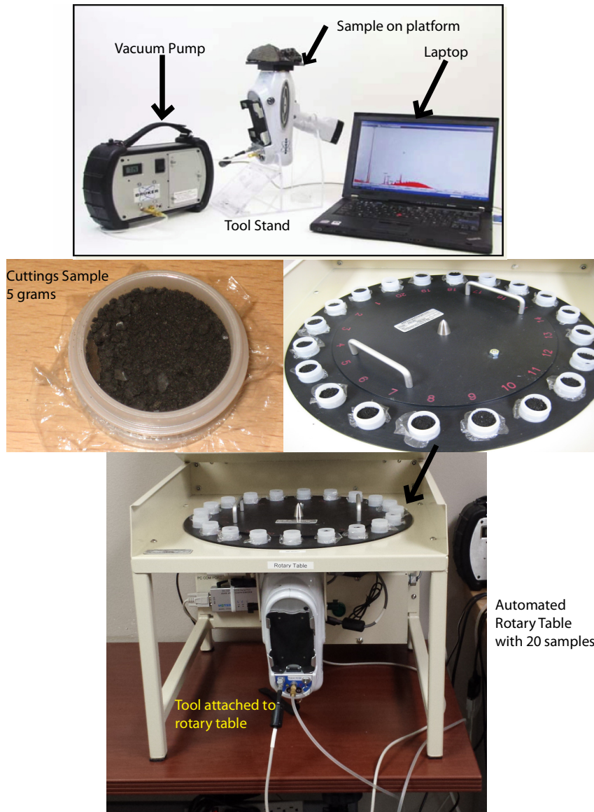
Figure 3.1 Rotary table set up at Pioneer's offices
