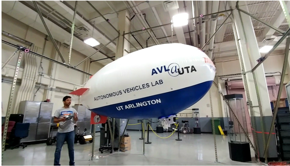
Figure 5.10. Airship inside the test area under motion capture system.
