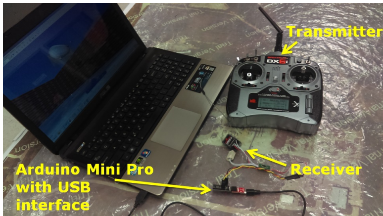
Figure 5.19. Hardware setup for the communication interface between the pilot and the airship flight simulator.
