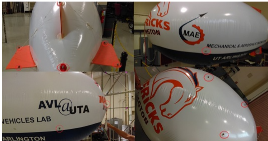
Figure 5.11. Marker placement on the airship hull.
