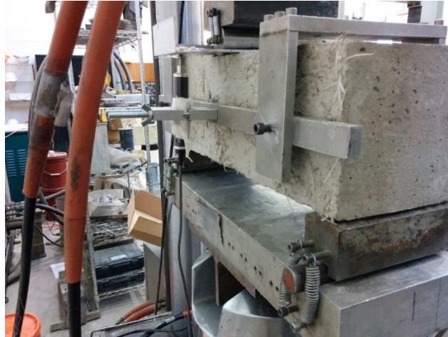
Figure 2-10 Arrangement for Obtaining the Net Deflection
