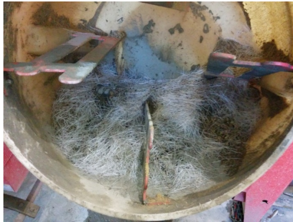
Figure 2-3 Fibers added to the Mixture
