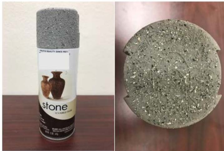
Figure 2-19 Spray Paint Used for Creating Speckle Pattern
