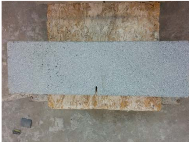
Figure 2-16 Notched Beam Specimen
