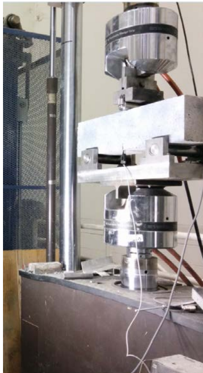
Figure 2-17 Test Setup of 3-Point Bending for DIC Validation
