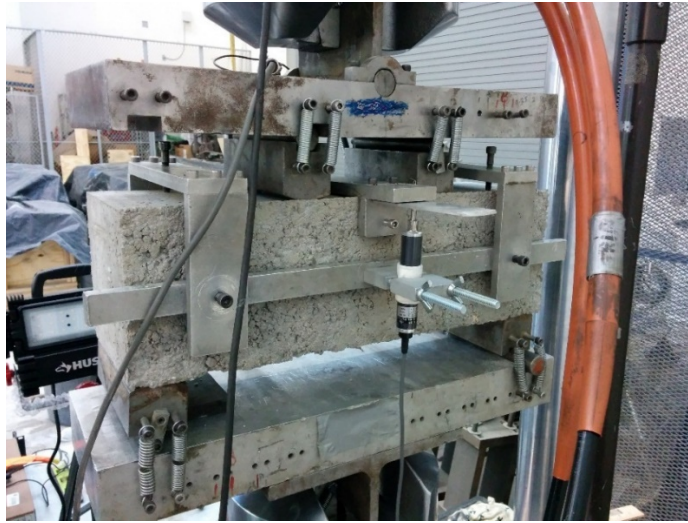
Figure 2-14 Arrangement to Obtain the Net Deflection
