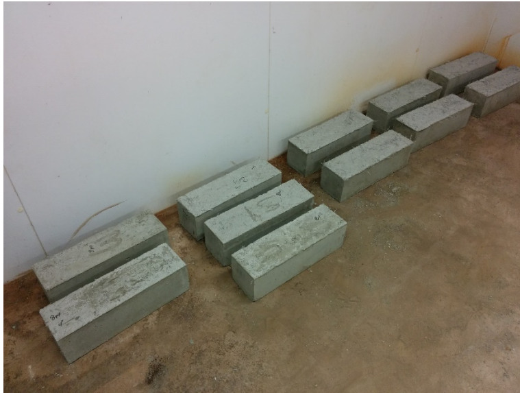
Figure 2-6 Beams Kept in the Curing Room for 28 Days
