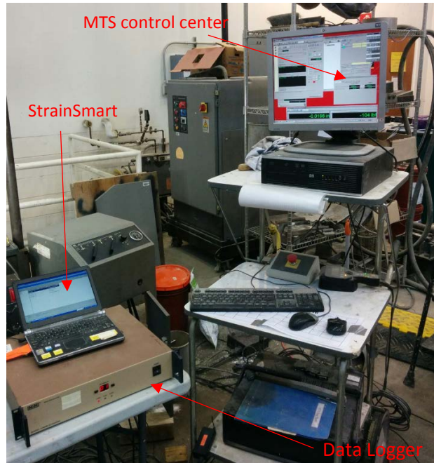
Figure 2-11 Data Acquisition System and MTS Control Center
