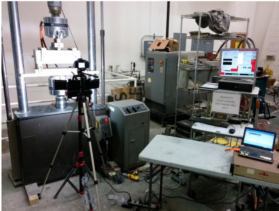
Figure 2-23 3-Point Bending Test Setup and DIC System
