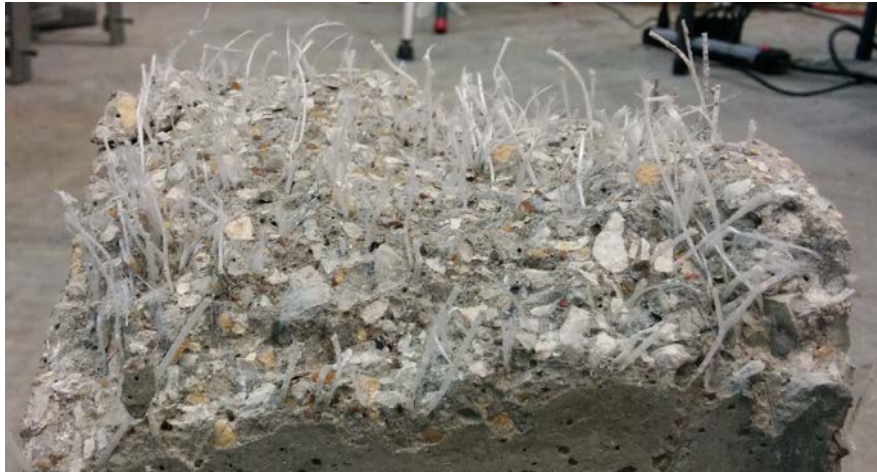
Figure 2-30 Beam Section after Total Failure (VF=1.04 %)
