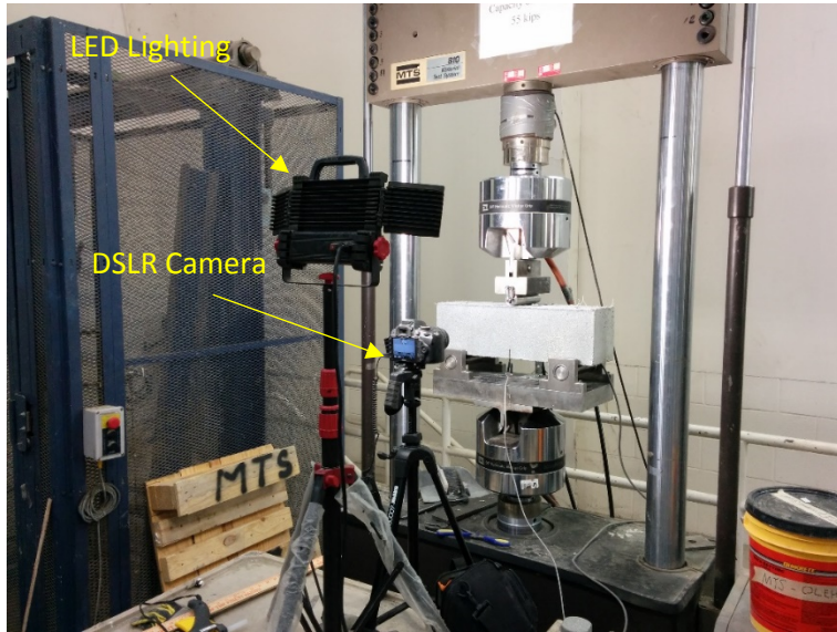
Figure 2-22 3-Point Bending Test Setup for DIC Validation - Camera and Lighting Device
