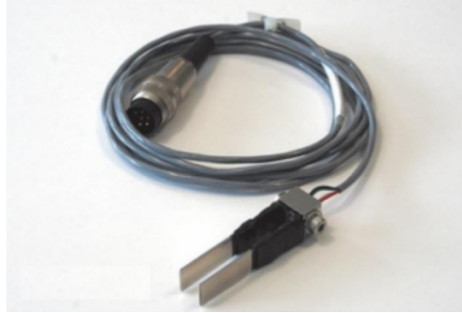
Figure 2-18 Clip Gauge Transducer (UB-5A)
