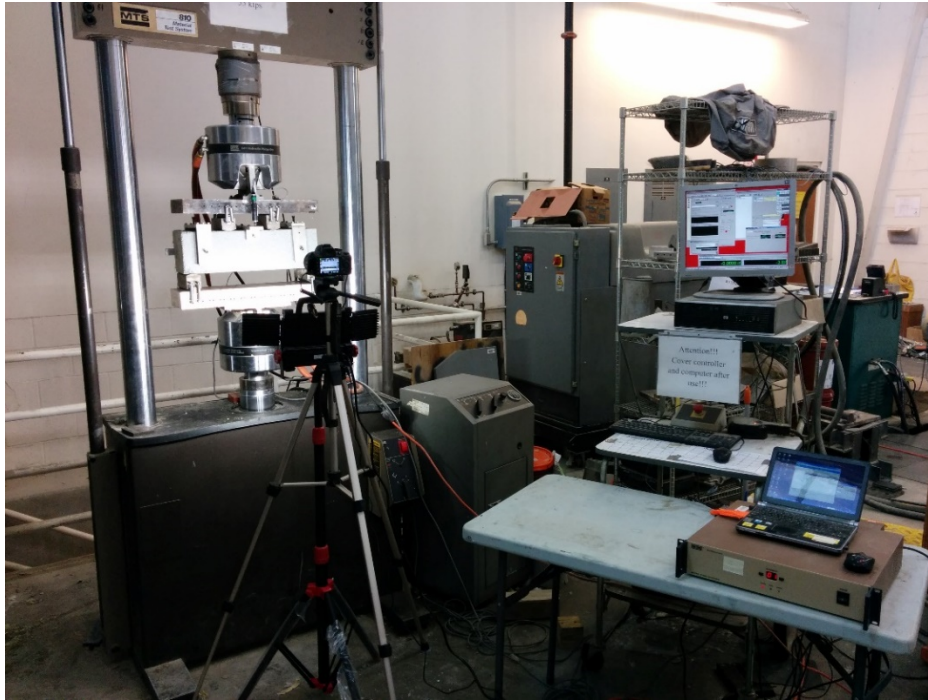
Figure 2-24 4-Point Flexure Test Setup and Camera Setup
