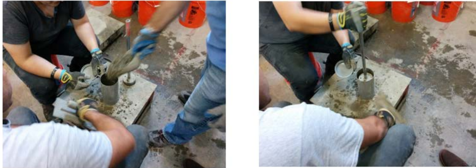
Figure 2-4 Casting and Compaction of Concrete Cylinders
