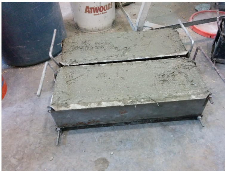
Figure 2-5 Beams after Casting
