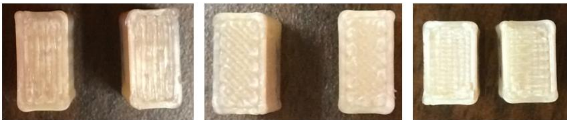
Figure 6-21 Broken cross section of 0°, +45°/-45° and 0°/90° oriented specimen
