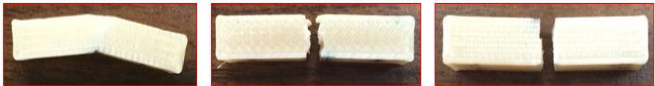
Figure 6-19 Break pattern of 0°, +45°/-45° and 0°/90° specimen under shear test
