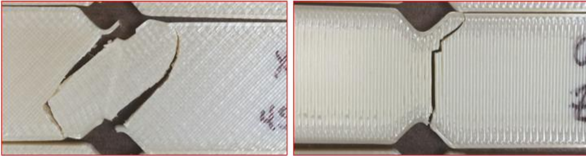
Figure 6.24. Fracture pattern of +45°/-45° and 90° raster oriented specimen
