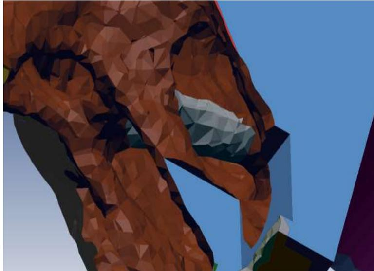
Figure 1-5 Noise and defects from the Topology Optimization results
