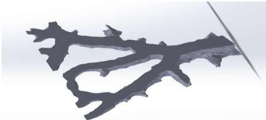
Figure 4-17 Material removal from Topology optimization result of the Missile Fin
