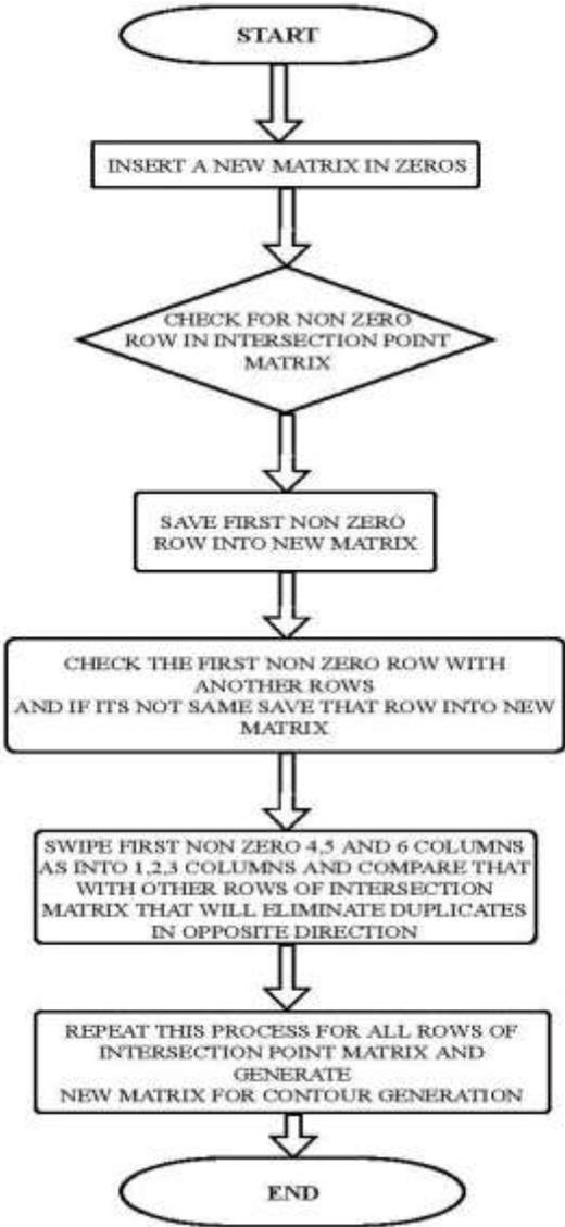
Figure 3-4 Step Flow chart to remove duplicate points
