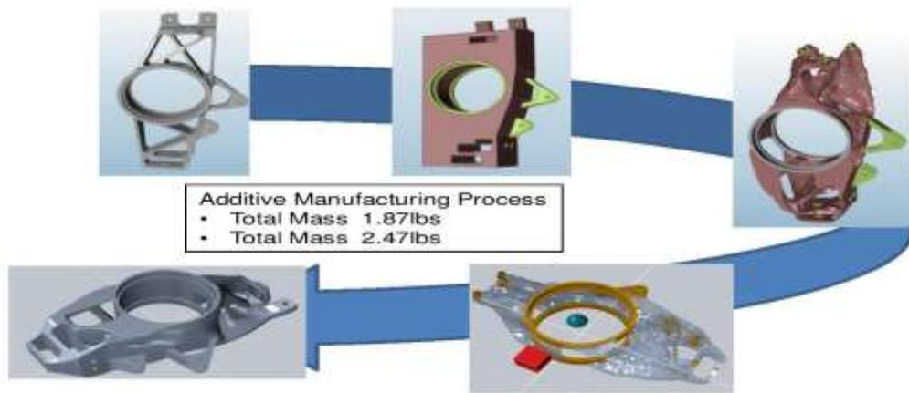
Figure 1-6 Topology Optimization Results for the Additive Manufacturing Process
