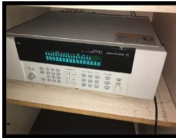
Figure 3-3 Data Acquisition System Agilent 34980A
