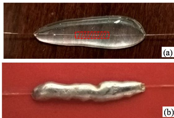
Figure 7-8 TFBG sensor coated with; (a) NOA-61 epoxy and (b) Solder paste
