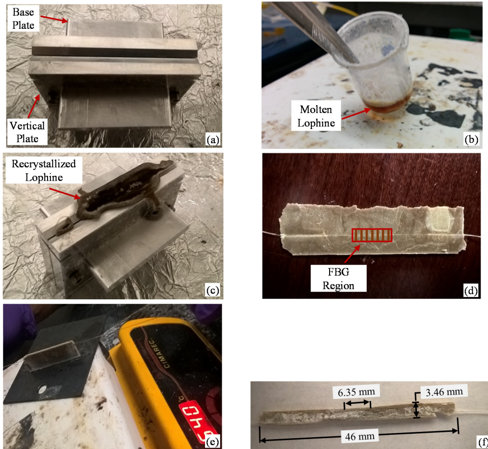
Figure 5-2. Coating Fiber Bragg Grating with recrystallized Lophine: (a) mold for thickness control; (b) melt Lophine in a beaker using a hot plate; (c) recrystallize Lophine in the mold; (d) recrystallized Lophine block with FBG encapsulated inside; (e) reduce the height of the recrystallized Lophine block using a heated plate; (f) final Lophine – coated FBG sample.
