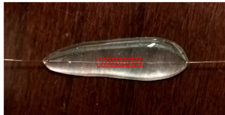
Figure 5-4. FBG sensor coated with NOA-61 epoxy.
