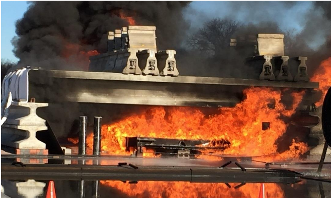
Figure 5-15 Uneven distribution of fire due to the wind
