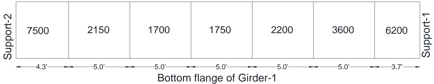
Figure 5-50 Hardness testing values of Girder-1 in psi
