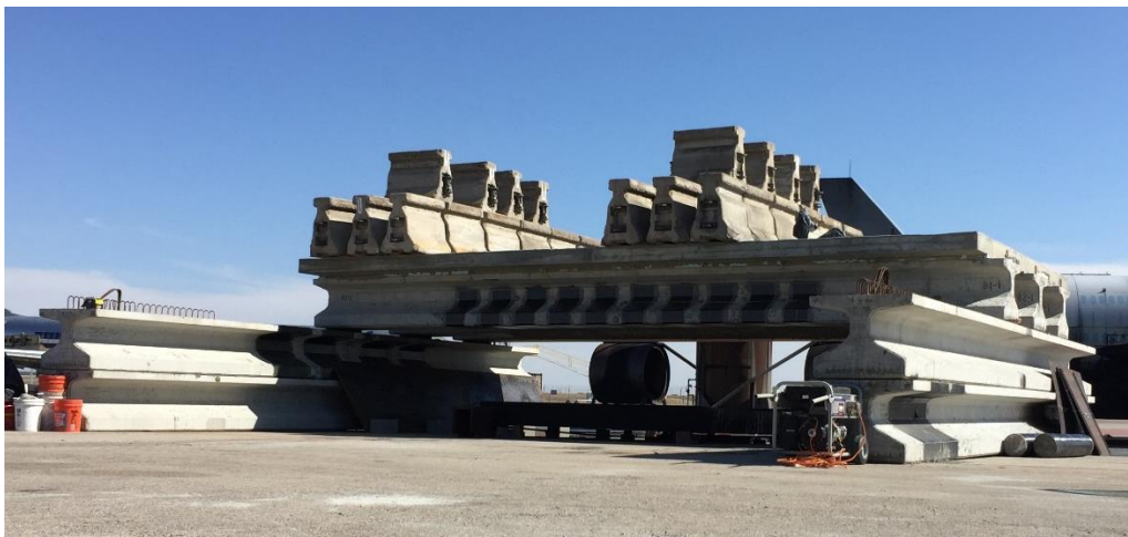
Figure 5-3 Test bridge loaded with the simulated AAASHTO HL-93 live load
