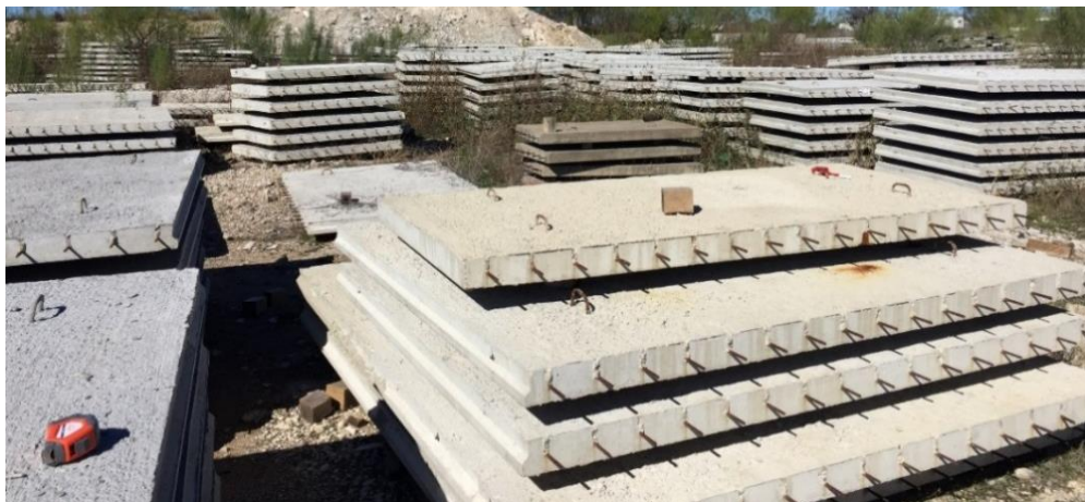
Figure 4-7 Prestressed concrete bridge deck panels
