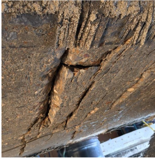
(a) Cracks on the bottom flange at mid-span
