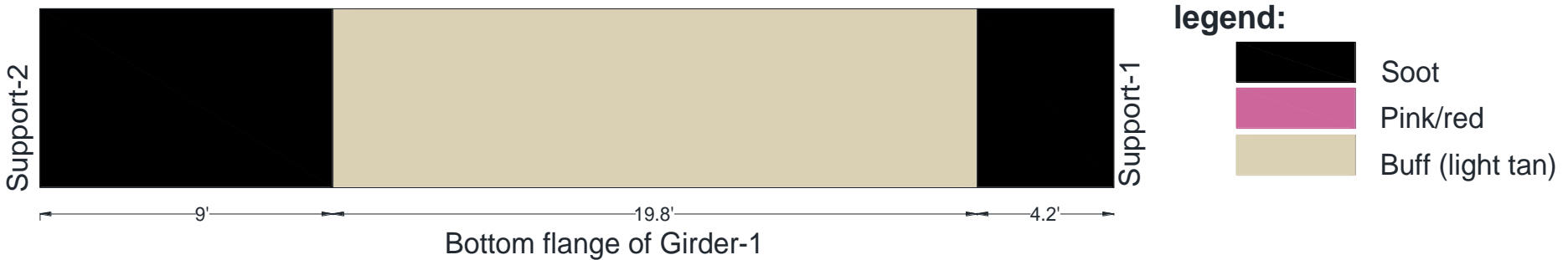
Figure 5-49 Visual inspection of Girder-1
