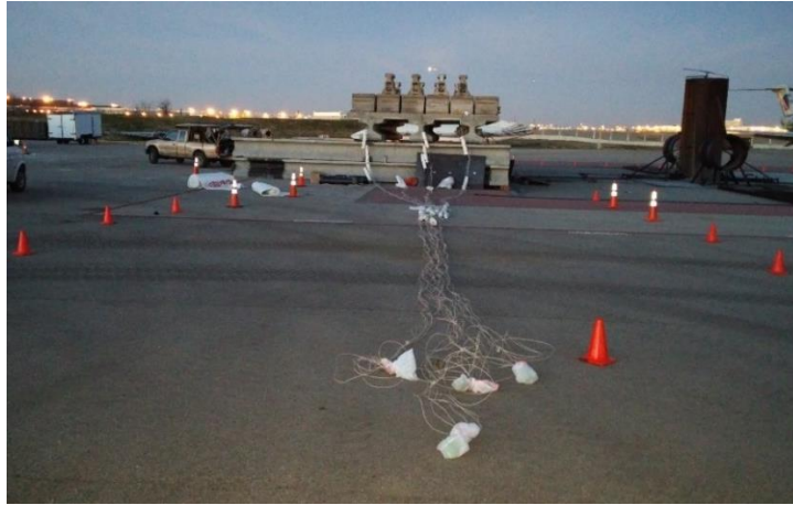
Figure 5-11 Thermocouple extension wire
