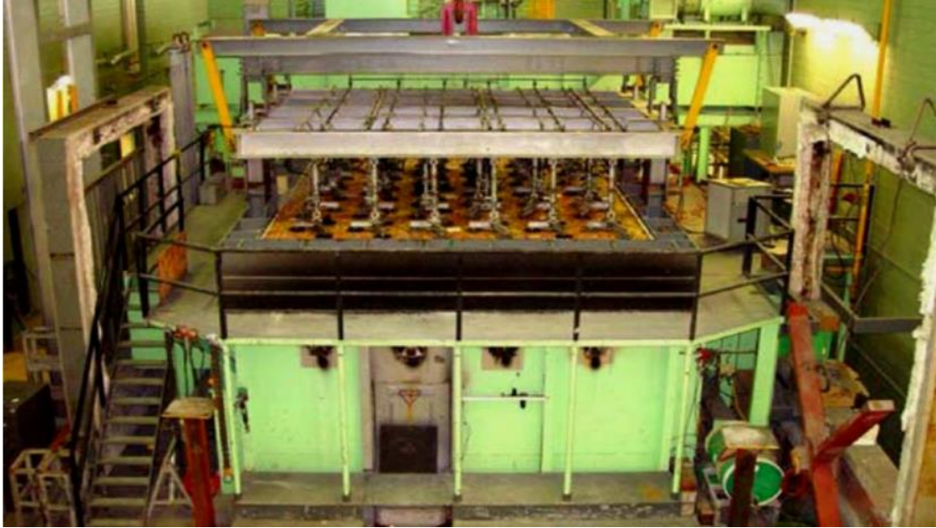
Figure 2-5 T-beams testing under ASTM E119 fire (Adelzadeh 2013)
