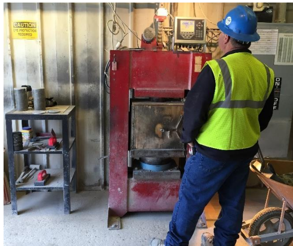
Figure 4-4 Testing to check if the release compressive strength of concrete is attained.
