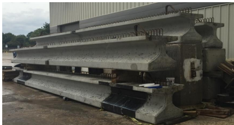
Figure 3-6 Previously tested TX28 Girders
