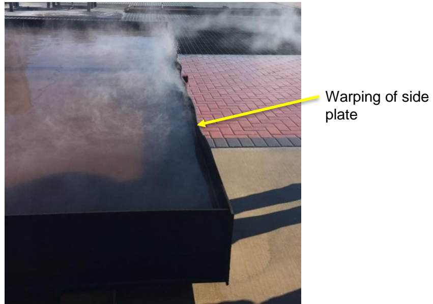
Figure 5-5 Warping of side of the pan
