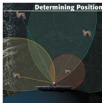
Figure 2.11 Localization using signals from four satellites [22]
