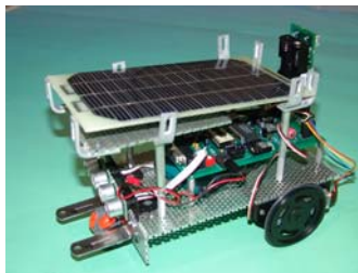
Figure 2.16 ARRIBOT-II prototypes, with a new chassis and a solar panel
