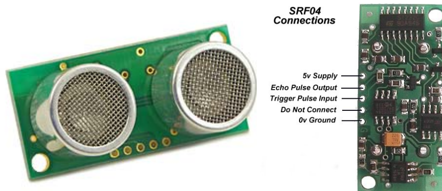
Figure3.8 Ultrasonic Transducer (SRF04)
