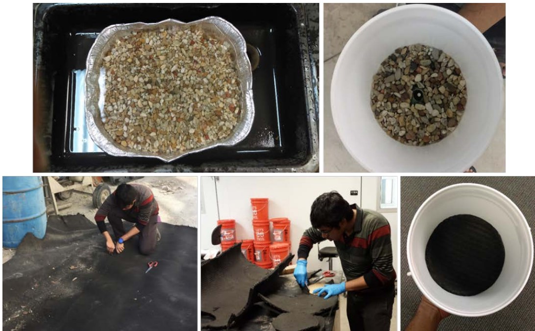
Figure 3.11 Pea gravel and geo-composite inside the reactor bucket
