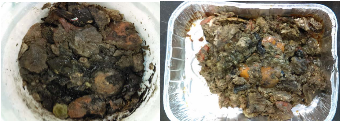
Figure 4.23 Waste inside reactor B8 after dismantling
