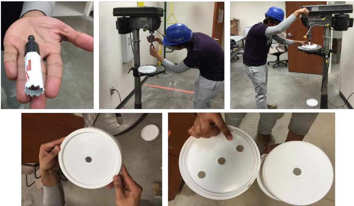
Figure 3.8 Drilling reactor bucket and lid
