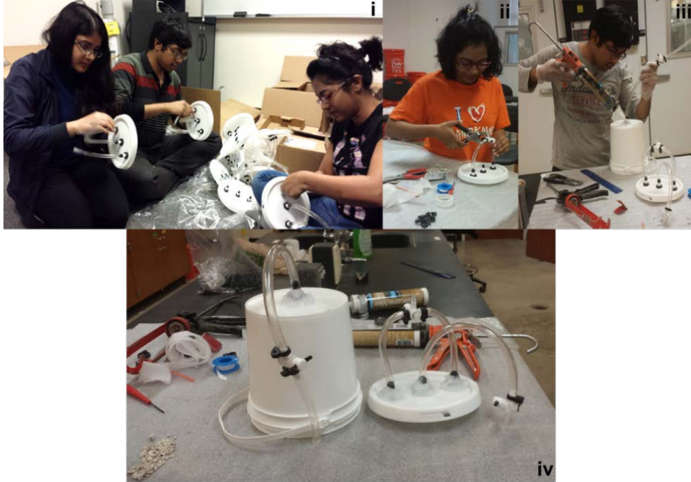
Figure 3.10 Tubing and valves connected using clamps and silicon sealant
