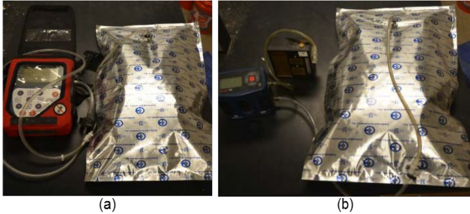
Figure 3.18 (a) Determination of gas composition by Landtec GEM 2000, (b) Gas volume determination with SKC grab air sampler and Defender 510
