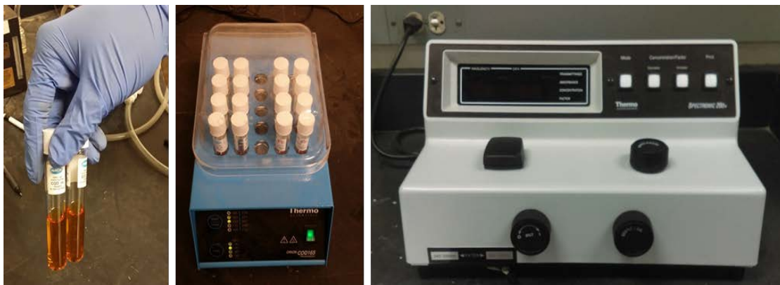
Figure 3.20 Chemical oxygen demand (COD) determination: (from left) COD vials, heating in digester, absorbance measurement by spectrophotometer
