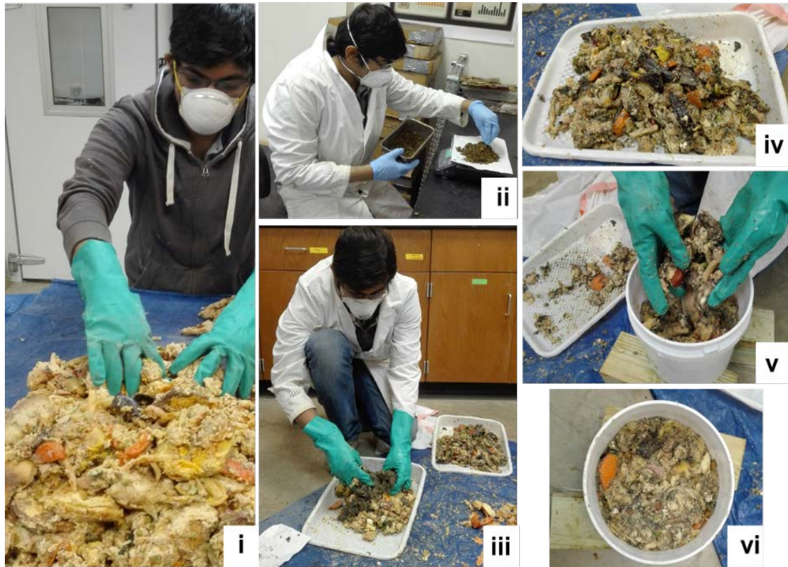
Figure 3.13 (i) Mixing waste; (ii, iii) weighing and mixing nutrient; (iv, v, vi) filling reactors
