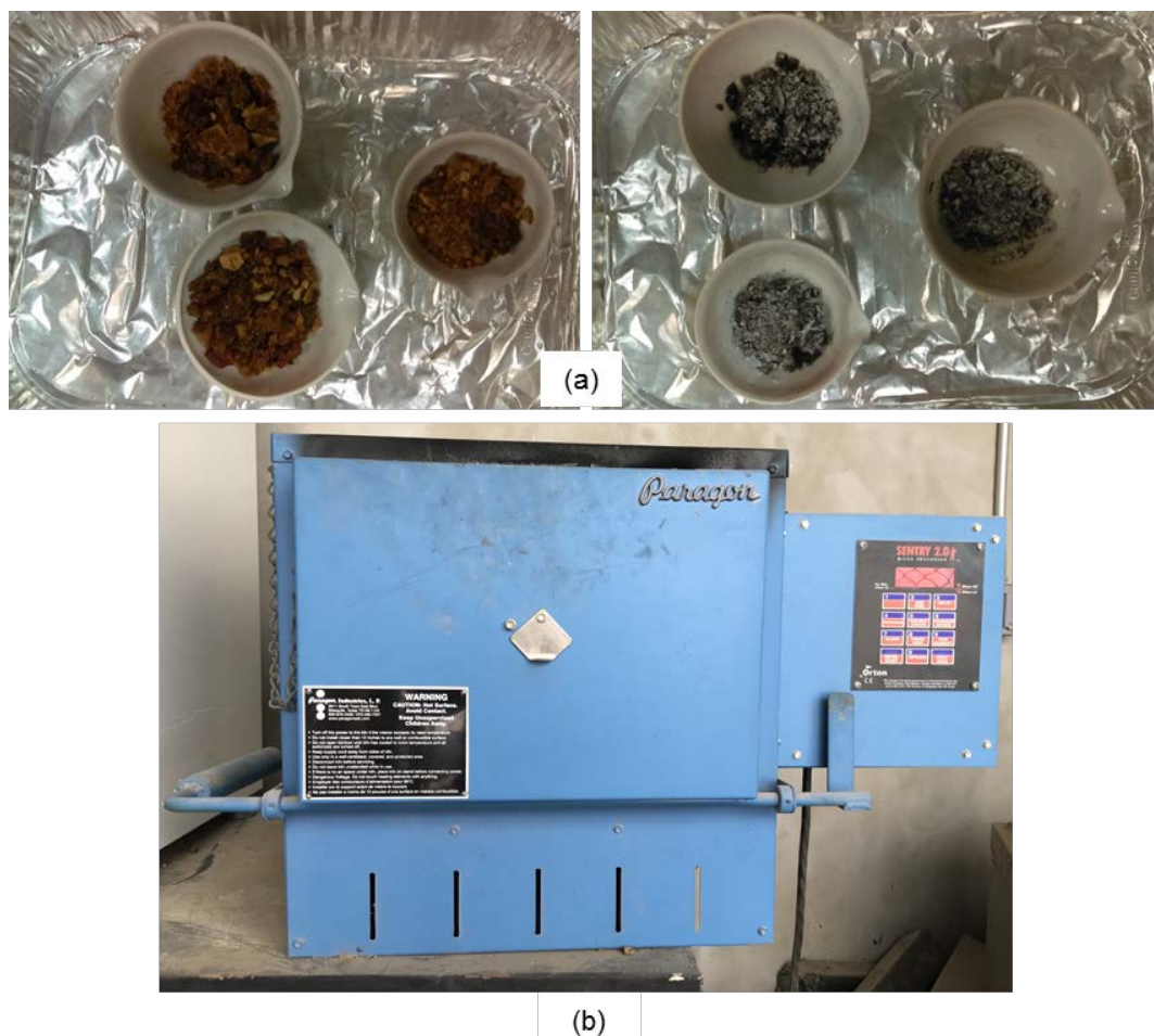
Figure 3.15 Volatile solids determination (a) samples before & after burning, (b) muffle furnace
