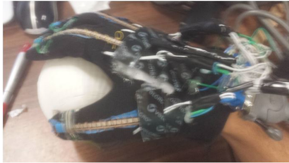
Figure 6: The sensor-embedded Master Glove that the user wears while grasping objects collects data for machine training.
