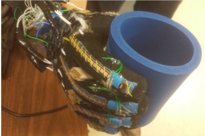
Figure 11: The spacers placed between the four fingers help to more accurately mimic the prosthetic hand.
