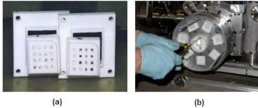
Figure 4.5 Picture of (a) cookie and (b) cartridge base used in the FPD detector.
