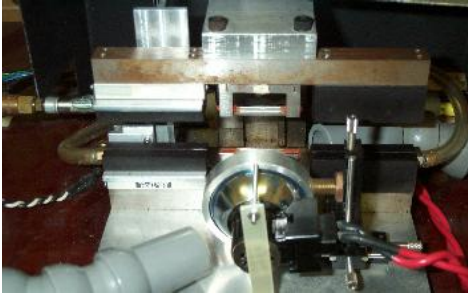
Figure 4.4 Picture of splicing machine used in production of FPD fibers.
