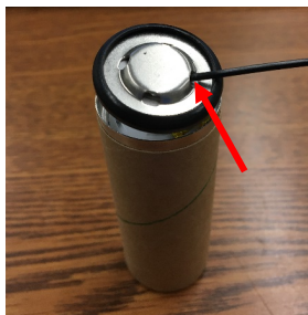
Figure 103: Copper reference wire fed through the top cap
