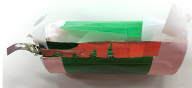
Figure 99: Picture of the jelly roll after the tape is cut and the roll unravels
