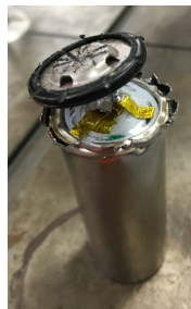
Figure 96: Picture of the top cap removed from the base
