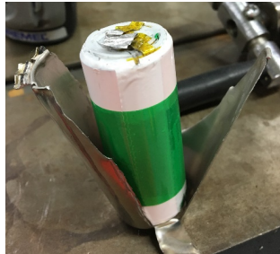
Figure 98: Picture of the side casing peeled back and the jelly roll exposed
