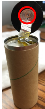
Figure 100: Picture of the hole drilled in the bottom side of the top cap
