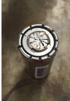
Figure 95: Picture of slits cut into the top cap
