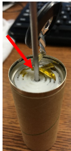
Figure 101: Metal rod inserted down the center of the cell
