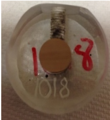
Figure 3-5 Polished 1018 steel sample
