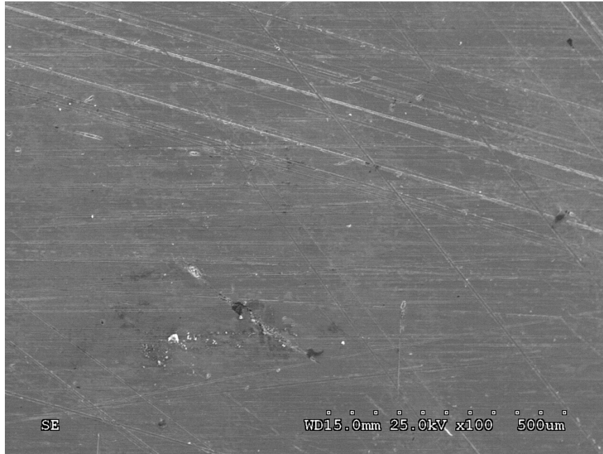
Figure 4-29 SEM image of the prepared 8620 steel sample
