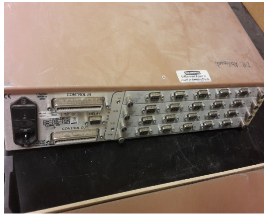
Picture 2-4, Vishay Scanner's Channels
