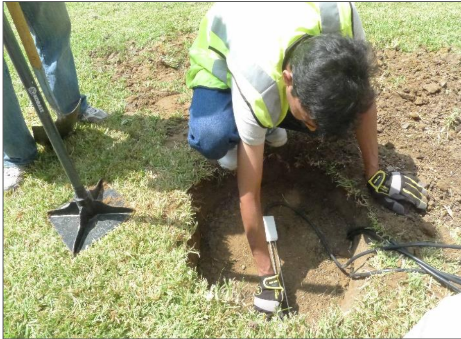
Figure 3-48 TDR sensor is placed at 0.05 m below the ground level facing the S direction as the orientation of the TDR Probe for each level need to be different.
