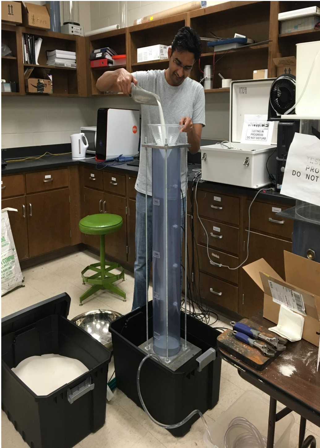
Figure 4-9 Pouring of ASTM Graded Sand through the means of funnel for equal compaction in the Soil Column Assembly
