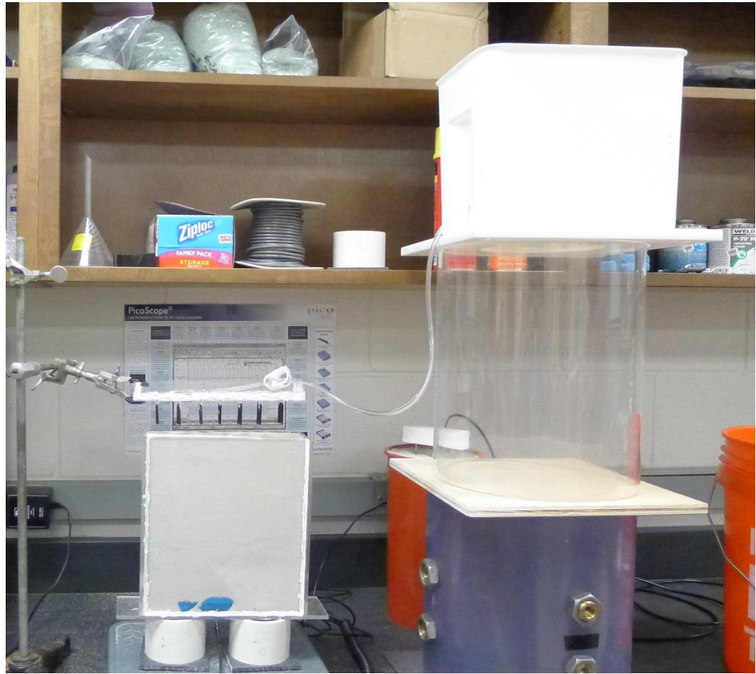
Figure 4-3 Infiltration Model for the Laboratory testing
