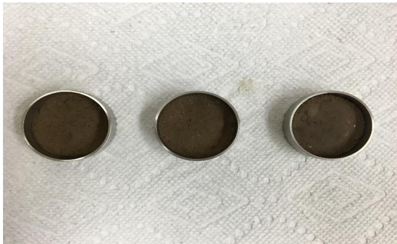
Figure 3-33 Samples prepared at different moisture content for testing with WP4C
