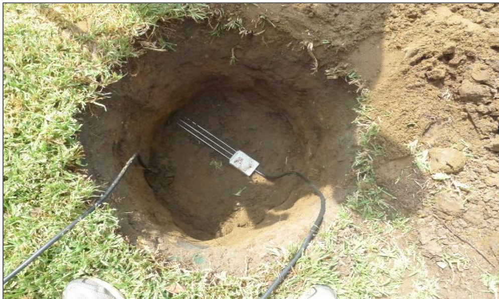
Figure 3-47 TDR sensor is placed at 1 m below the ground level facing the N-W direction.
