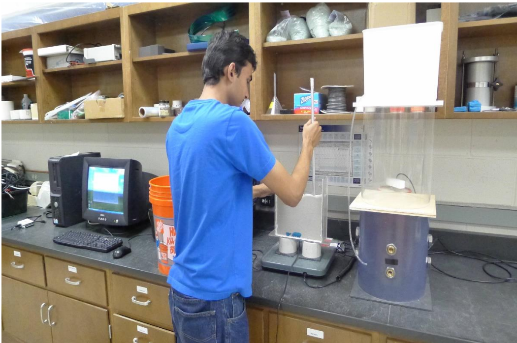
Figure 4-2 Compaction being applied to the ASTM Graded Sand
