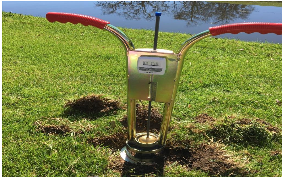
Figure 3-69 Turf Tec Infiltrrometer installed at Station 3 TDR location
