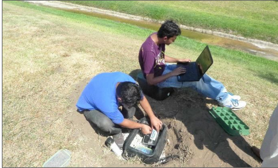
Figure 3-44 The sensors are validated and set at fixed interval for recording the data
