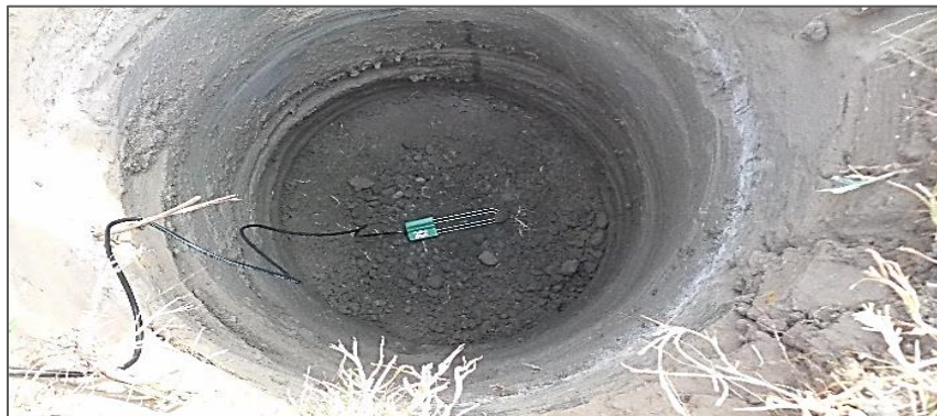
Figure 3-39 TDT sensor placed at 1 m depth after leveling the ground
