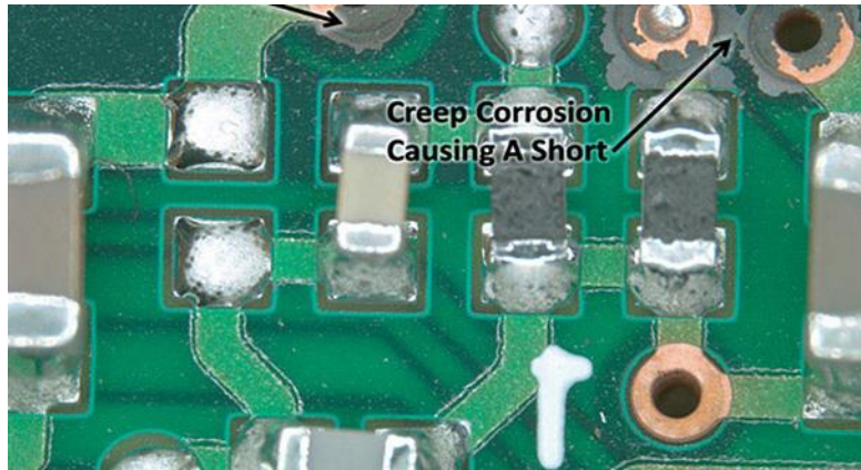
Figure 2-2; Creep Corrosion Causing short Circuit
