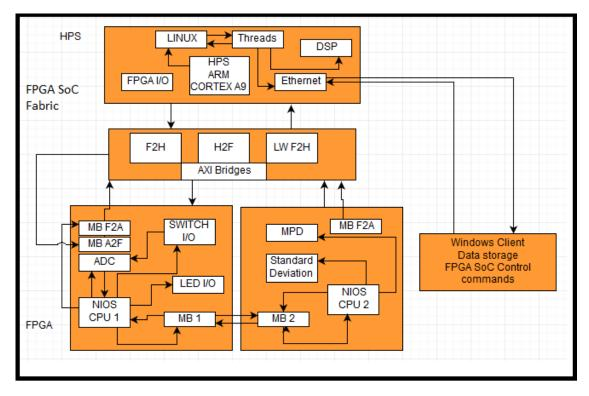
Figure 5.7 Complete Soc architecture for data acquisition, processing and Ethernet
