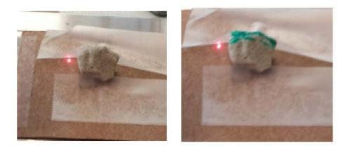
Figure 6.6 Laser measurements on a marked and unmarked aggregate.
