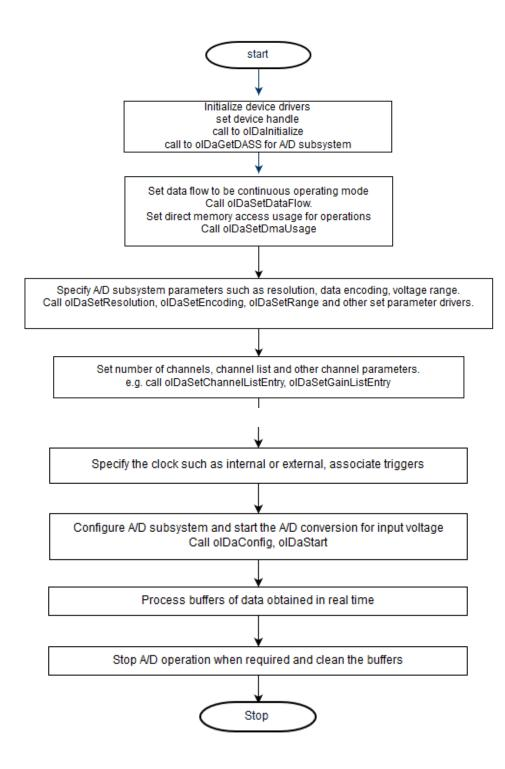
Figure 3.9 Data acquisition control flow using DT9816 module
