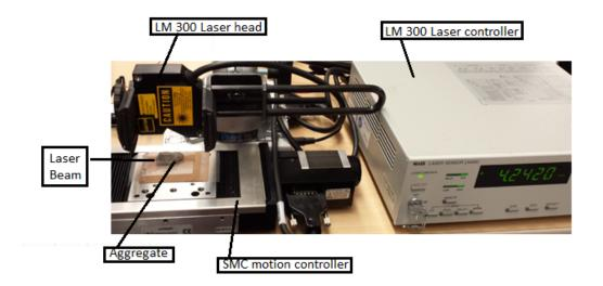
Figure 6.2 LM300 with SMC Motion control system
