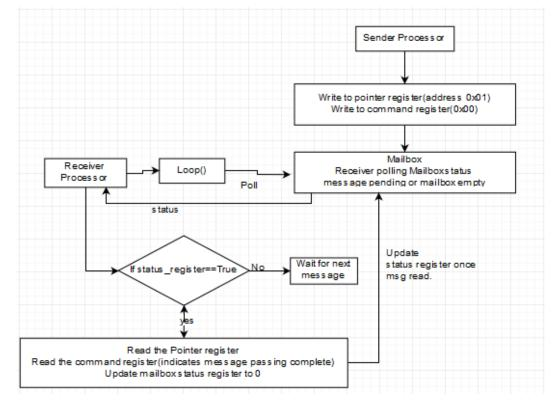
Figure 5.12 Flow diagram of Mailbox core send and receive message.
