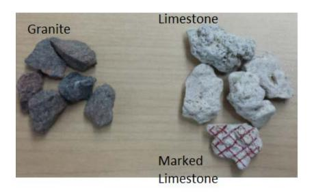
Figure 3.15 Granite, limestone sample and a marked aggregate for analyzing the laser color immunity.
