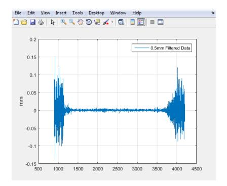
Figure 3.19 Surface estimation using high-pass IIR filter on scanned data.
