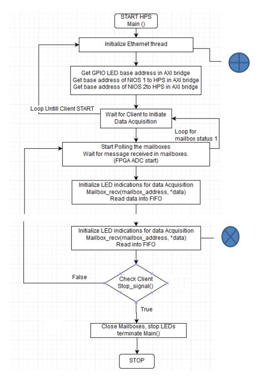
Figure 5.15 Flow chart for HPS multithreaded processing and Ethernet communication. -61 -
