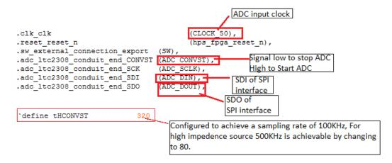
Figure 5.3 Design Verilog entry for ADC module.
