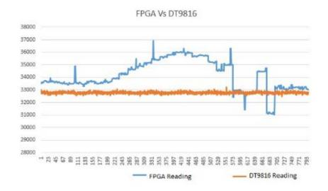
Figure 6.4 Comparison of Level of detail between 800 points obtained from DT9816 board and FPGA board.
