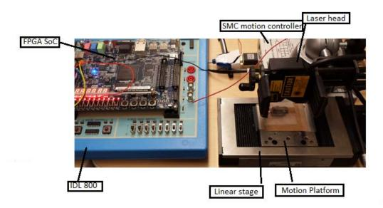
Figure 6.3 Complete FPGA Texture measurement instrument
