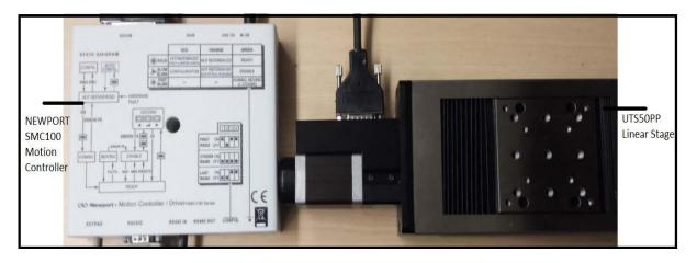
Figure 3.21 Newport SMC100 controller and UTS50PP linear stage
