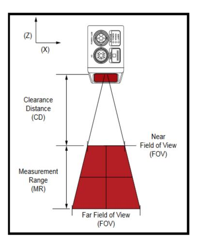
Figure 3.3 Measurement terminology for Line laser. [6]
