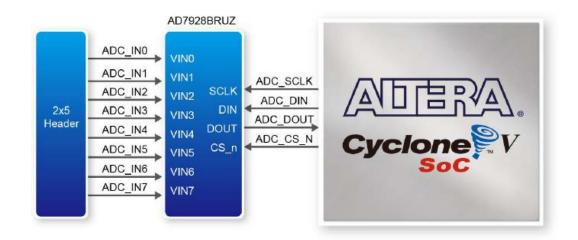
Figure 4.5 ADC LTE2308 and FPGA interface with connectivity pins. [15]
