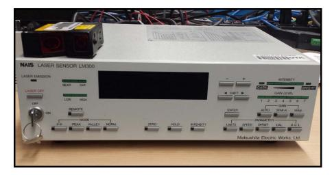
Figure 3.5 NAIS LM 300 laser sensor and controller
