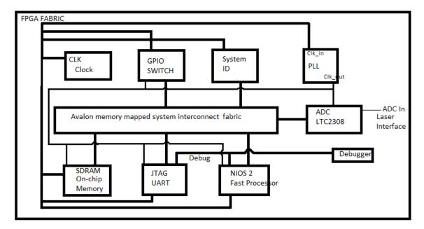
Figure 5.1 Block diagram of ADC data acquisition on FPGA fabric
