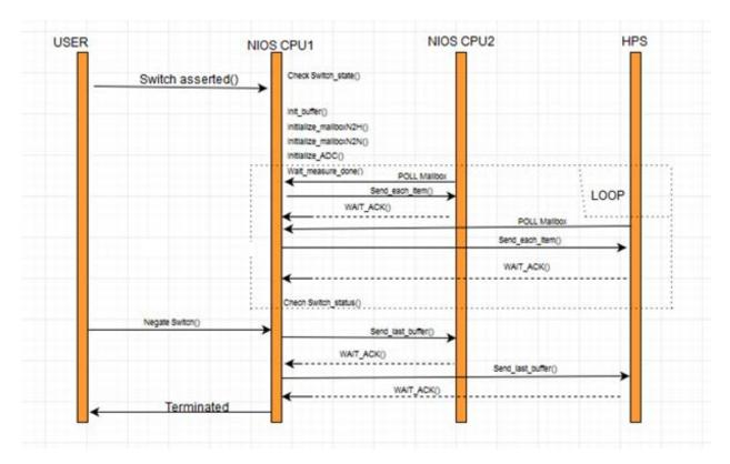
Figure 5.14 Time sequence diagram for FPGA side operations.
