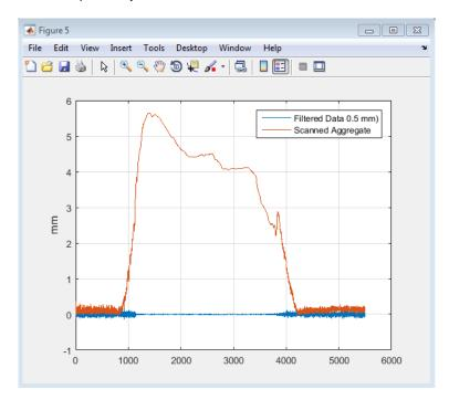
Figure 3.18 Data and IIR filter plot for granite sample.
