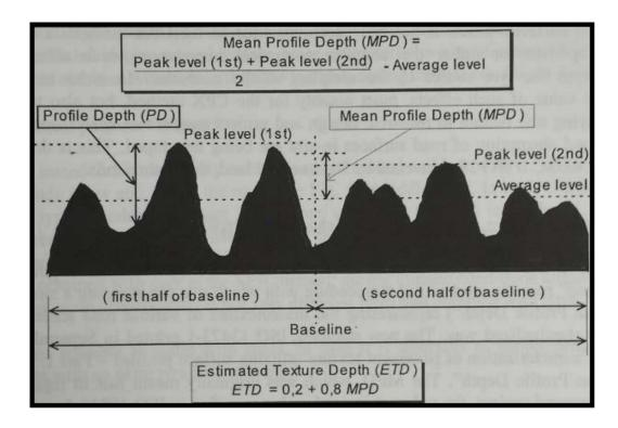
Figure 1.3 Profile Depth and Mean Profile Depth calculations. [12]
