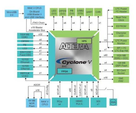
Fig. 1.2 Block diagram of Altera ARM based SOC chip. [11]
