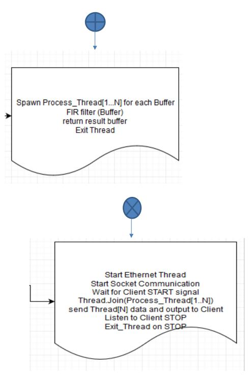
Figure 5.16 Flowchart for HPS multithreaded processing and Ethernet communication
