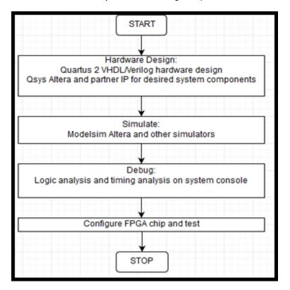
Figure 4.2 Hardware design flow diagram.
