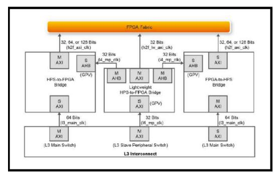
Figure 4.4 AXI Bridge interconnect for FPGA- HPS on System on Chip [15]
