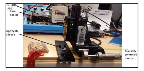
Figure 3.12 Laboratory setup for test equipment.
