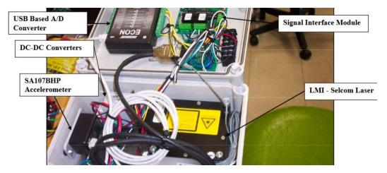
Fig 1.1 A laser based road profiler. [10]
