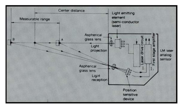
Figure 3.1 Laser triangulation technique for NAIS LM 200 Lase sensor [5]
