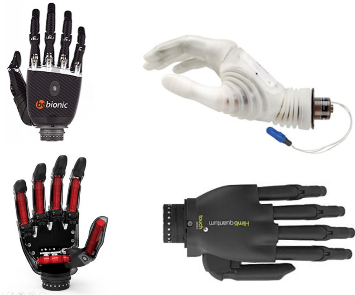
Figure 2.4 Several State of the Art prosthetic hands. Top Left: bebionic hand, image from [31]. Top Right: Otto Bock Michelangelo Hand, image from [32]. Bottom Left: Vincent Hand, image from [35]. Bottom Right: TouchBionics iLimb Quantum, image from [33].
