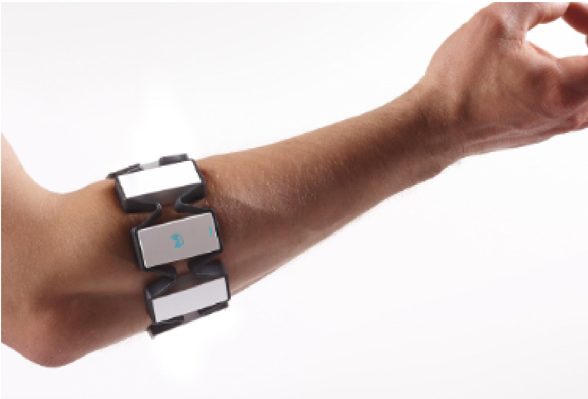
Figure 2.9 The Myo armband is a gesture input device utilizing eight EMG sensors as well as accelerometers.
