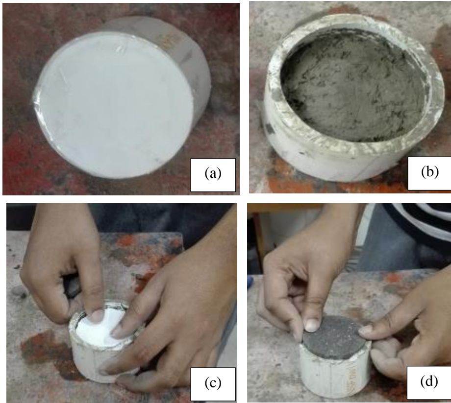
Figure 3-4 Placing of soil sample
