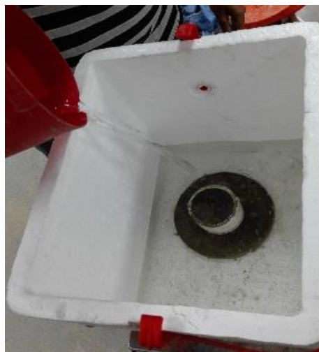
Figure 3-5 Saturating the sample by adding water
