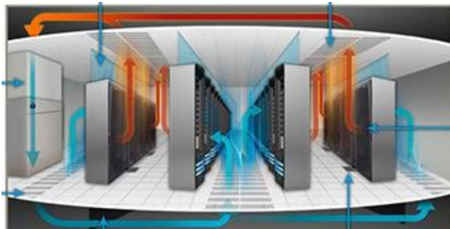
Figure 1-2 Schematic diagram of flow of air in cooling data center.
