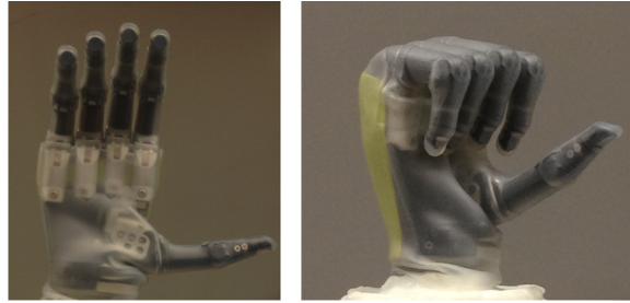
Figure 4.14: The prosthetic device in the fully open (left) and fully closed (right) positions.
