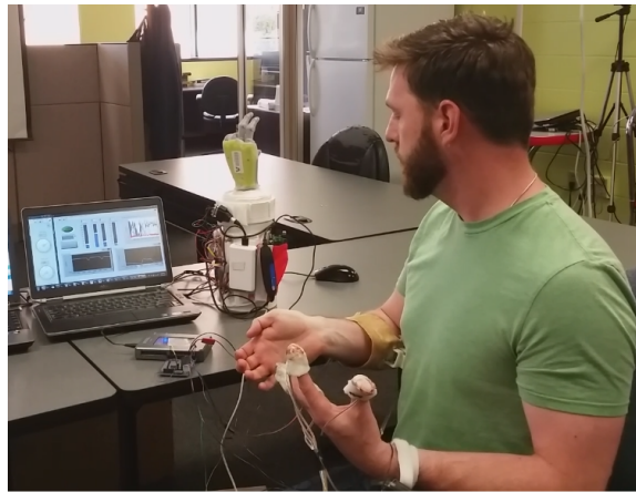
Figure 4.13: The experimental setup, including contact sensors, healthy limb socket, and prosthetic device. The subject can be seen performing a hand extension action with their right hand.
