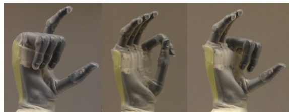
Figure 4.16: Prosthetic Device in each of the three closed grip configurations. Index Finger Point (Left) Lateral Grip (Middle) Modified Lateral Grip (Right)
