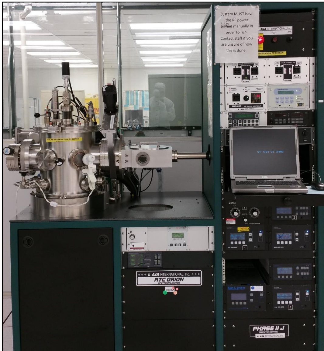
Figure 4.10. The AJA ATC 5 Orion UHV sputtering system for deposition of dielectric (non-conducting) thin films, at Schimadzu Institute: Nanotechnology Research Center (UTA) .
