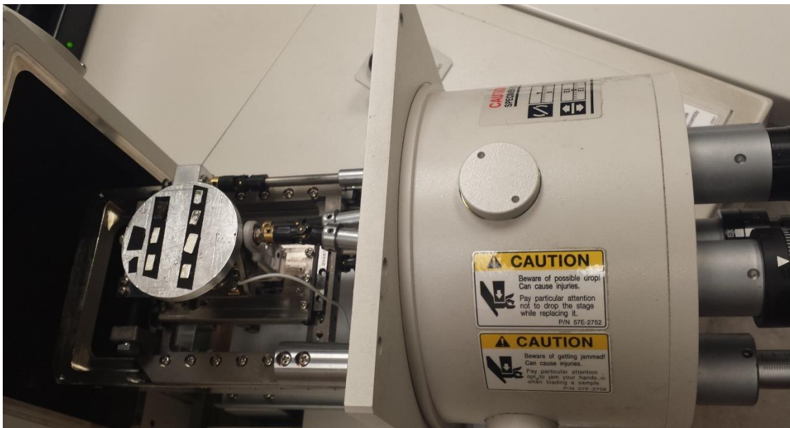
Figure 4.29 Several composite samples of LC and dispersion of Au NPs loaded together on the sample stage for imaging in S-3000N SEM
