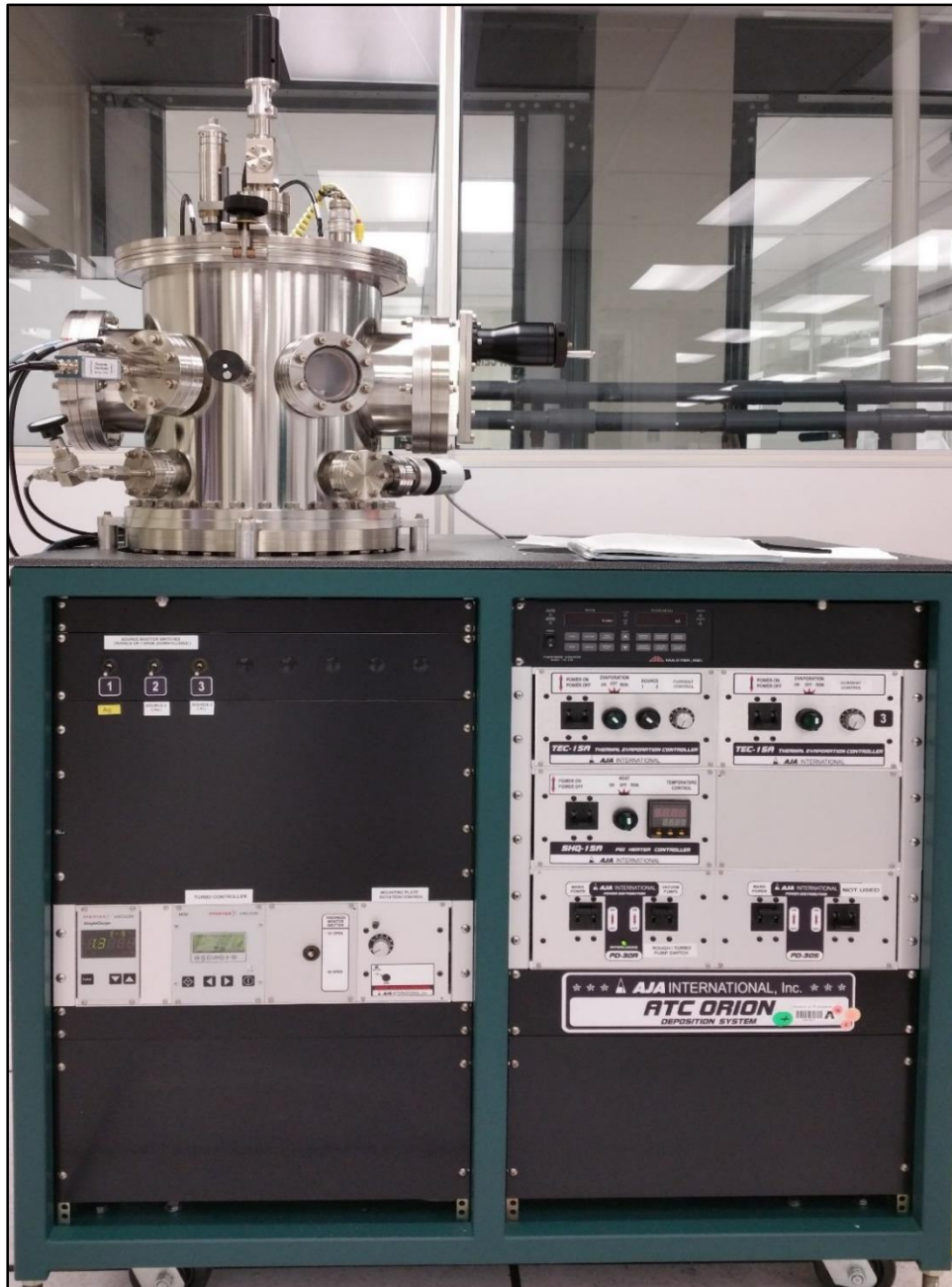
Figure 4.8. AJA ATC ORION Series thermal evaporation system facilitated by three separate thermal evaporation sources, at Schimadzu Institute: Nanotechnology Research Center (UTA) .
