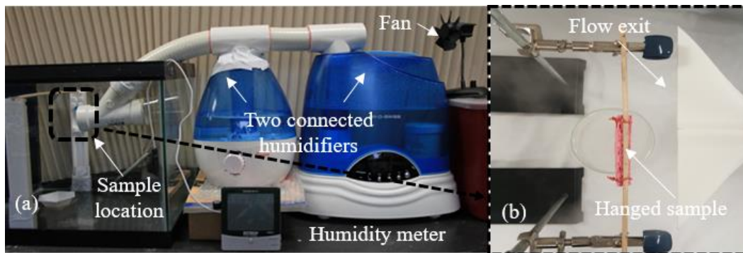
Figure 1: (a) Experimental setup for the water collection and (b) closed-up view of flow exit and sample location.
