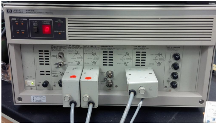
Figure 4-1: Picture of HP 4142B modular dc source/monitor with High Power SMUs (HPSMUs) and Ground Unit (GNDU) connections.
