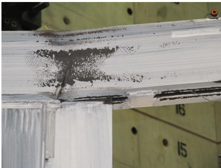
Figure 4-12 Fracture at 1.5% story drift ratio in STMF-2C8-1
