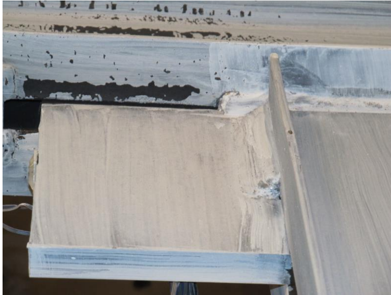
Figure 4-12 Fracture at 1.5% story drift ratio in STMF-2C8-1
