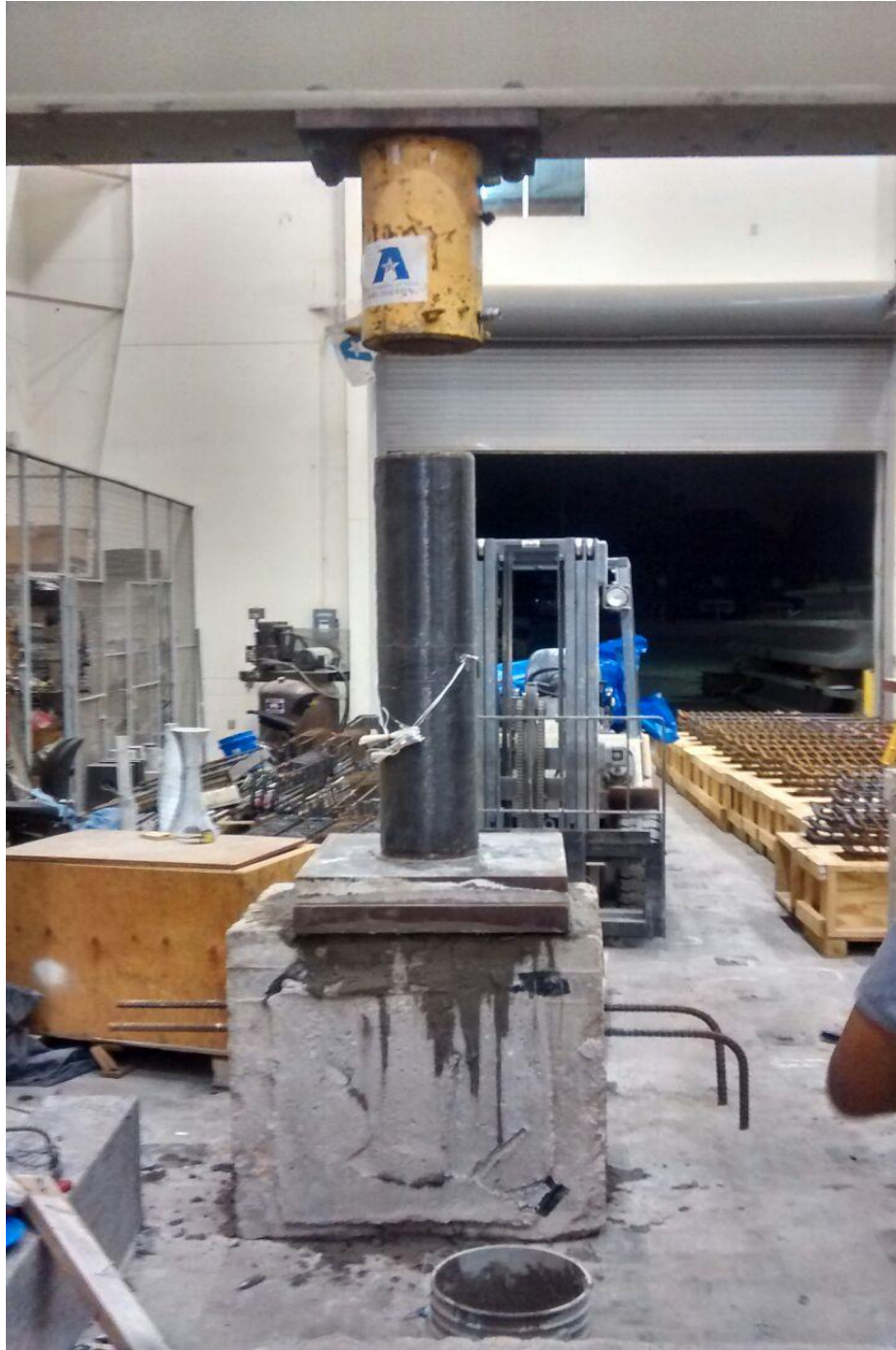
Figure 6 Picture showing the test setup of the column at Civil Engineering Laboratory, University of Texas at Arlington
