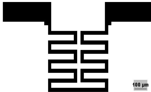
Figure 3-4 (a) Mask showing design of ITO heater and (b) mask showing hydrophilic opening, used in photolithography for device fabrication
