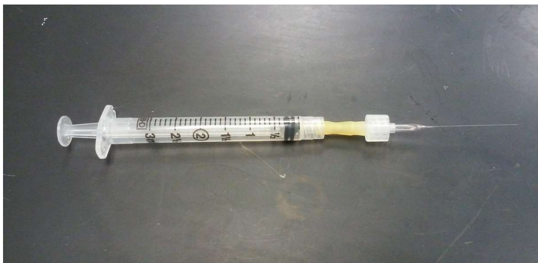
Figure 12 : Syringe with quartz capillary tube
