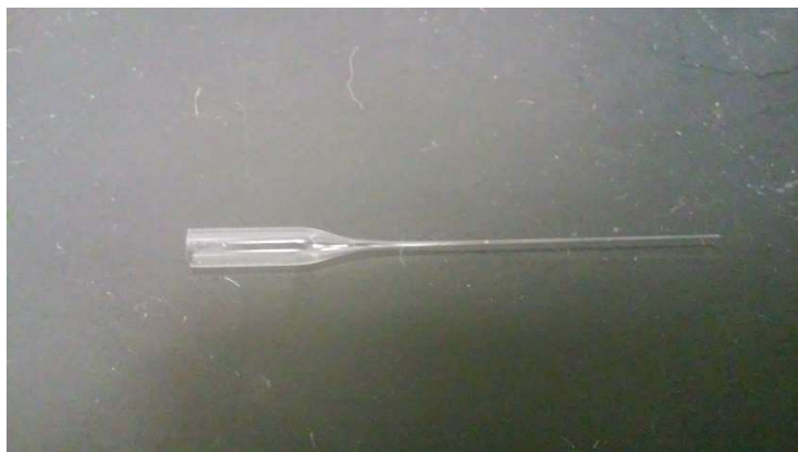
Figure 11 : Thin walled quartz capillary tube
