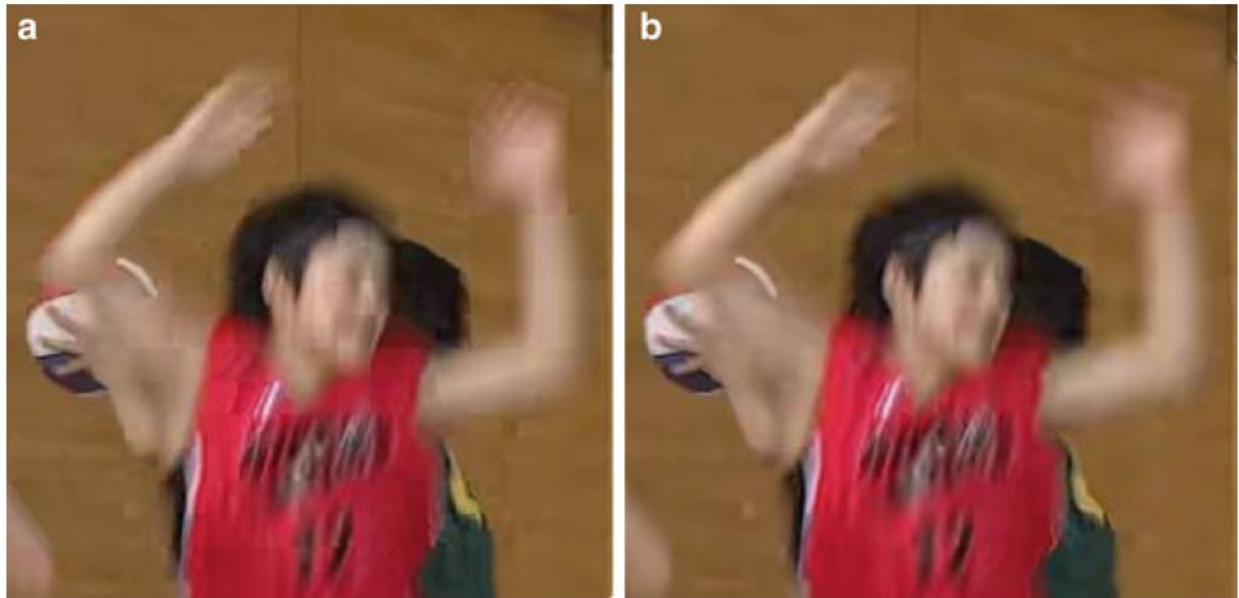
Sequence BasketballDrive , Random Access, QP32: (a) deblocking turned off, (b) deblocking turned on
