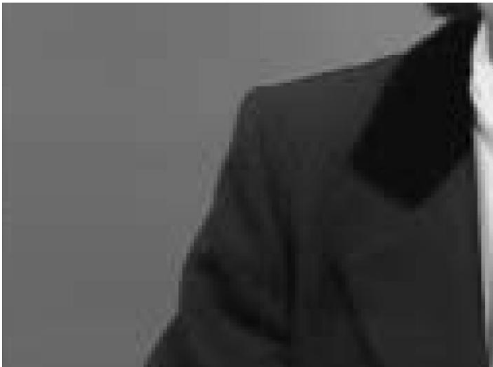
Figure 45. Example of the ringing effect in a sequence coded at a relatively high bit-rate. Most prominent along the edge formed by the upper-arm in the scene [16]
