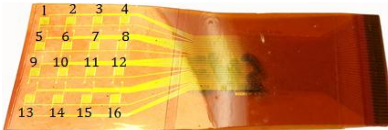
Figure 4-15 Sensor array with markings
