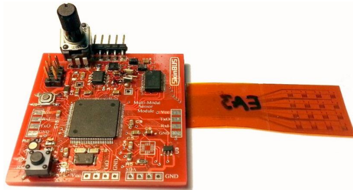
Figure 3-24 sensor array connected with the SkinCell
