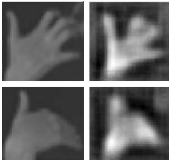
Figure 7-2 Gray scale image and its inverse HOG image as proposed by [14]
