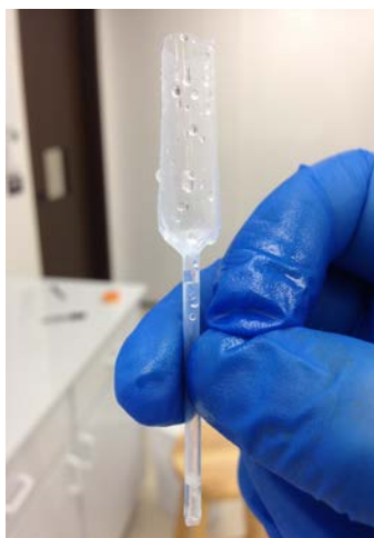
Figure 3-2 125 \mu\text{L} Teflon column, photo taken in UTA Clean Lab by the author.
