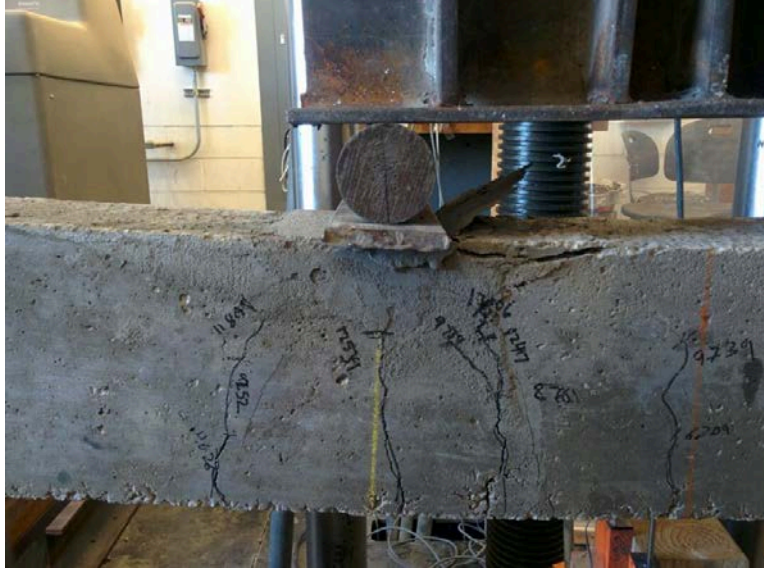
Figure 35 Failure Mode for the control beam
