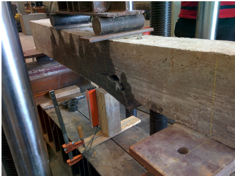
Figure 36 Failure mode for the strengthened beam without anchorage
