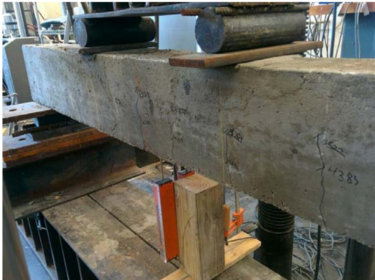
Figure 31 Crack pattern for control
