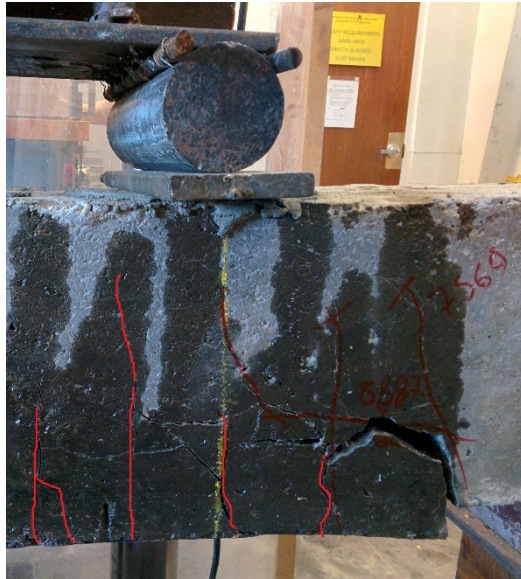
Figure 37 Failure mode of strengthened beam with Anchor bolt
