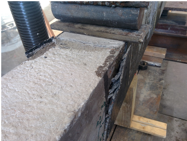
Figure 38 Failure mode of the strengthened beam with U-Wrap
