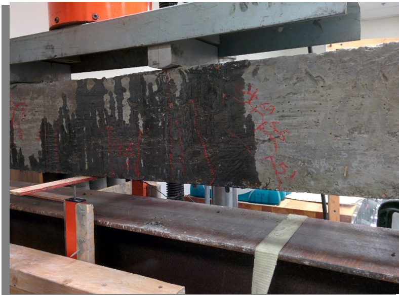
Figure 32 Crack pattern for Beam Strengthened without anchorage
