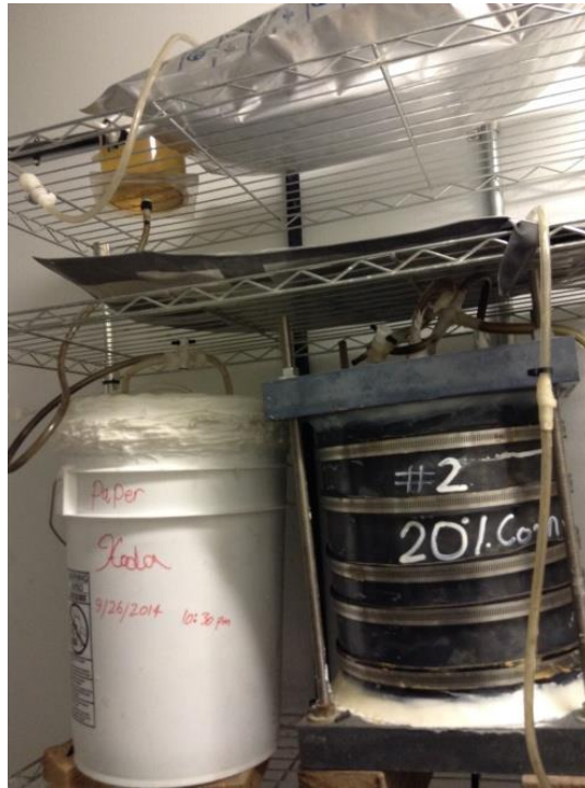
Figure 3-17 Gas collection bag at top of white reactor (with my name Hoda on it), and leachate recirculating glass at top
