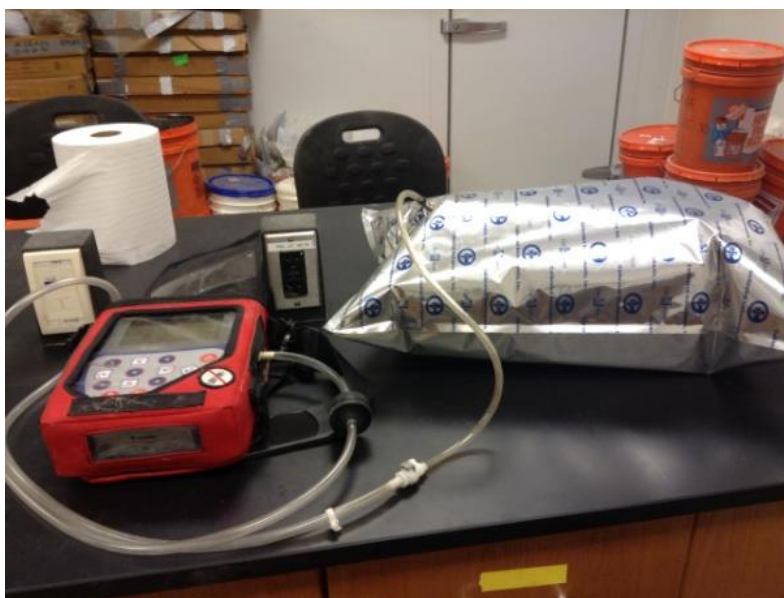
Figure 3-20 Gas generated from reactor; gas composition measured by using Landtec
