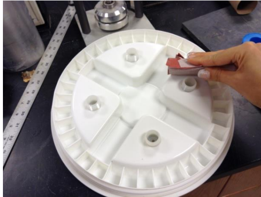
Figure 3-4 Using emery on gamma seal for making a rough surface for better application of sealant
