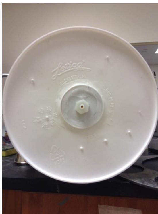
Figure 3-8 Transparent sealant was applied at the bottom of reactor
