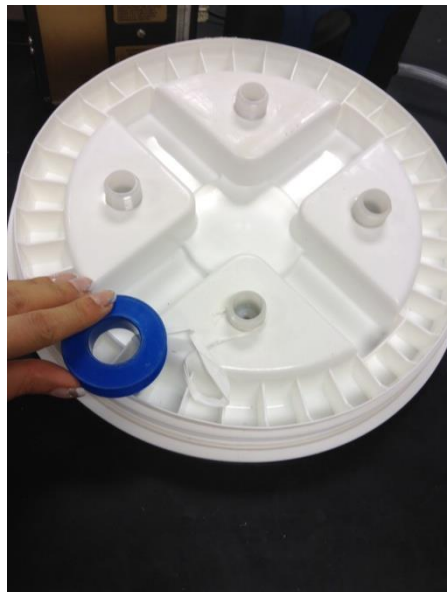
Figure 3-5 Using plastic tape around threaded adapter to ensure there is not any leakage
