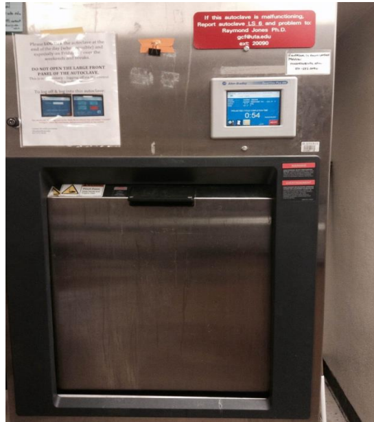
Figure 3-26 Oven used for autoclaving media
