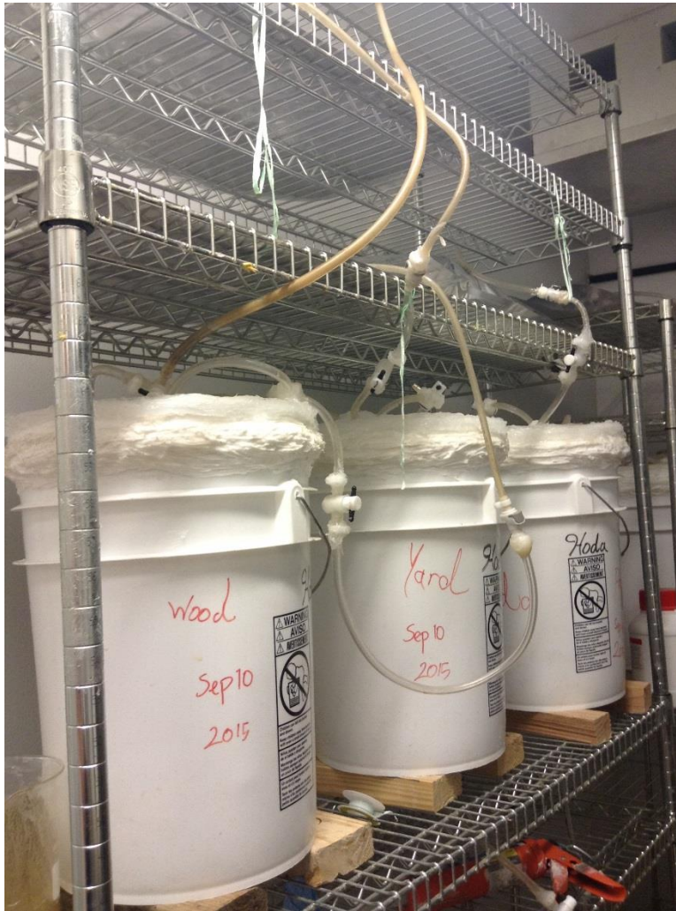
Figure 3-35 Hot room operation of another 3 reactors with termite gut microbes
