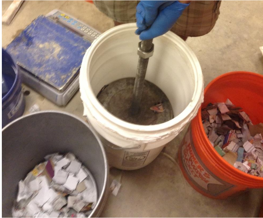
Figure 3-15 Compacting of waste in reactors by a compacting tool
