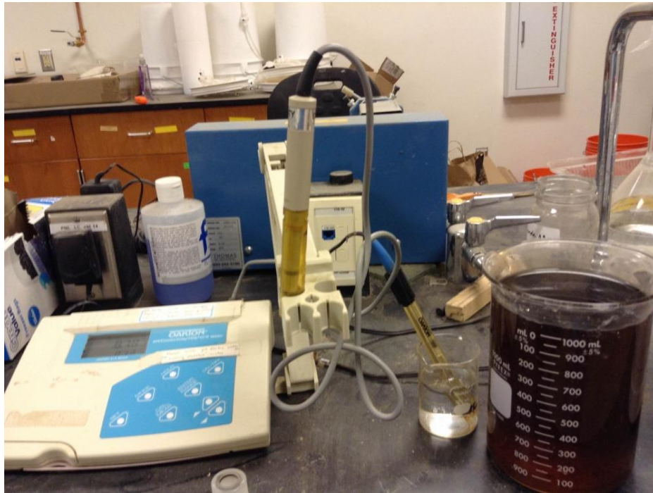
Figure 3-19 pH meter for measuring pH of Leachate
