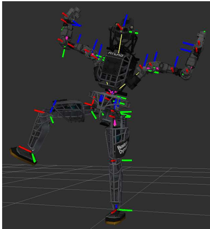
Figure 8.7. The Atlas robot kinematic structure with left foot as base link.
