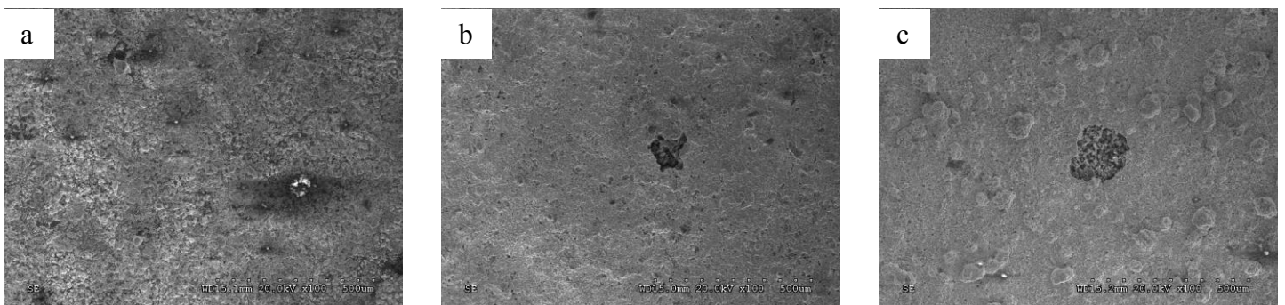
Figure 6-35. Surface SEM micrograph of EPP deposited Ni on Al at 185 V and (a) 30 s, (b) 60 s, and (c) 90 s after anodic polarization measurements.
