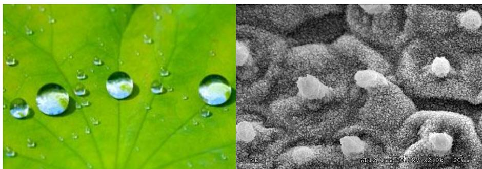
Figure1-2:(a)Water droplet on a lotus petal,[Image Source: www.rsc.org] (b) SEM image of lotus surface, clearly showing the hierarchical structures covered with wax crystals.
