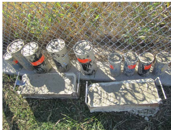
Figure 4-18 Photograph of typical CLSM specimen for compressive strength test
