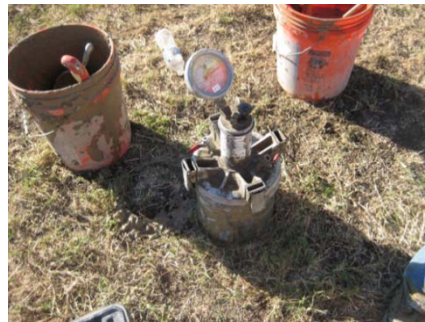
Figure 4-19 Air content test was conducted on the CLSM material
