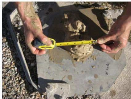
Figure 4-20 Spread test conducted on the CLSM to quantify the flowability of the CLSM
