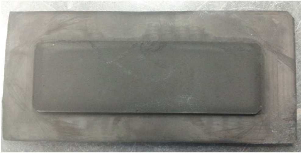
Figure 25 Top part machined by micro mill
