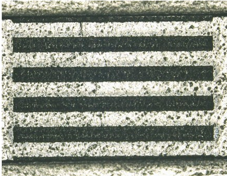
Figure 28 Microchannels machined on the mold using laser (before cleaning)
