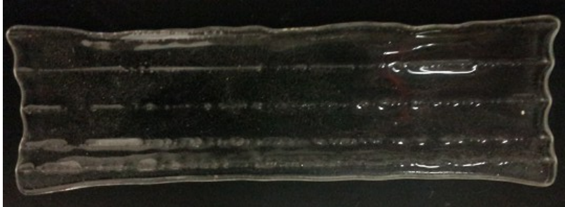
Figure 20 Improvement step 1 using SFG TM mold in a kiln
