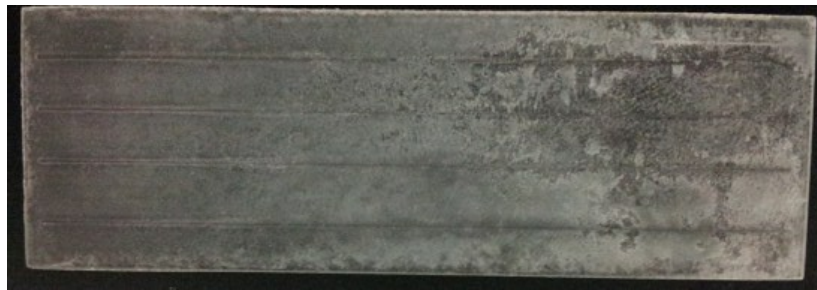
Figure 19 Glass slide resulting from using GLASSMATE-HT™ mold
