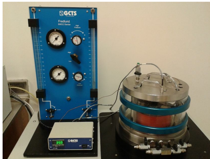
Figure 4-16. Final assembly of the temperature controller system before the start of a test.
