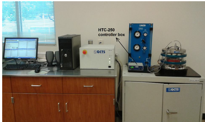
Figure 4-4. Panoramic view of the Thermo-servo/suction controlled Ring Shear Apparatus
