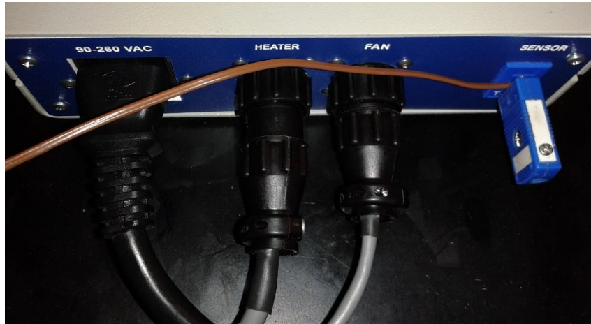
Figure 4-8. Backside of the HTC-250 controller box during a test.
