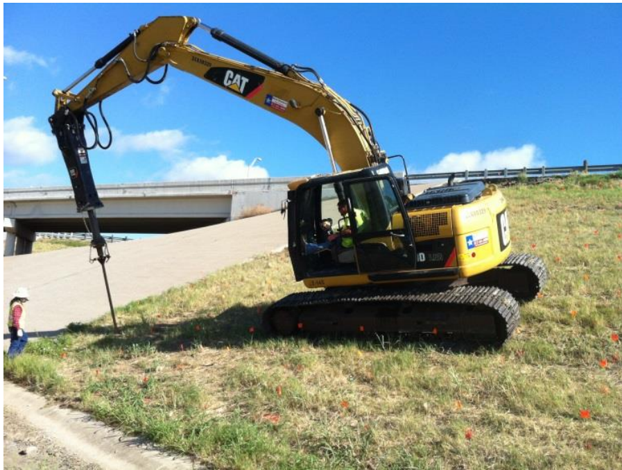
Figure 4-17 Conventional rig with hydraulic hammer
