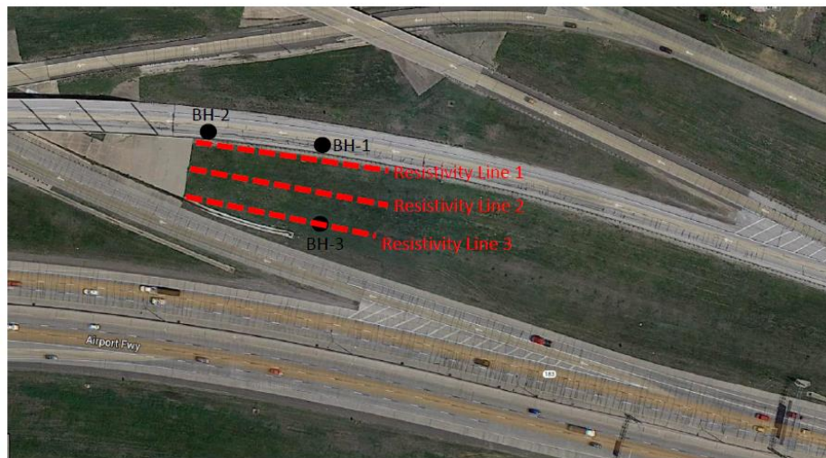
Figure 3-10 Borings and Resistivity Imaging location
