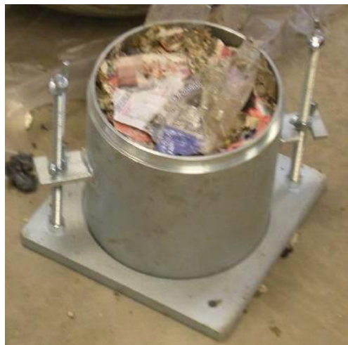
Figure 3-11 Fully compacted MSW in compacted mold
