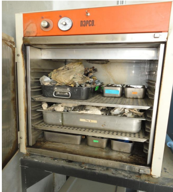
Figure 3-9 Samples placed in oven for Determination of Moisture content
