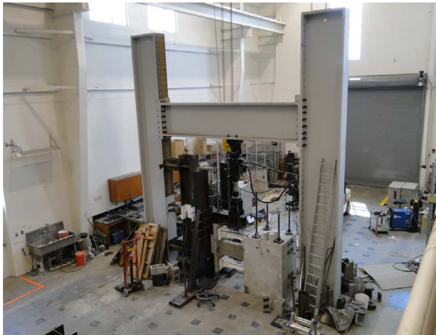
Figure 3.11 Test setup for the coupling beam experiments
