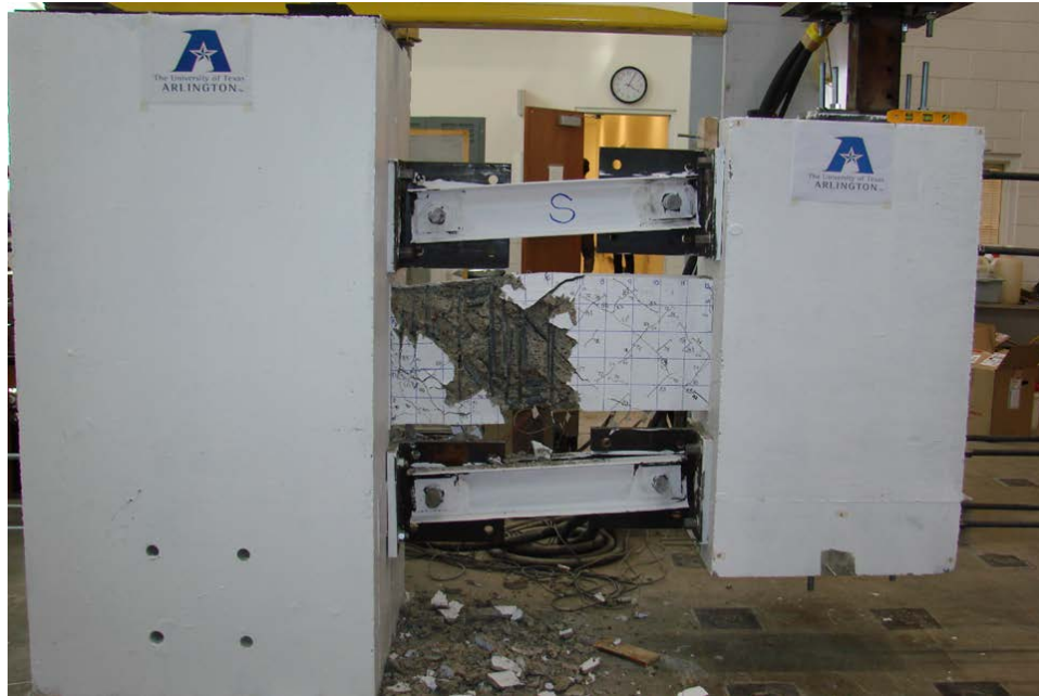
Figure 4-2 Torsion failures for CB-1
