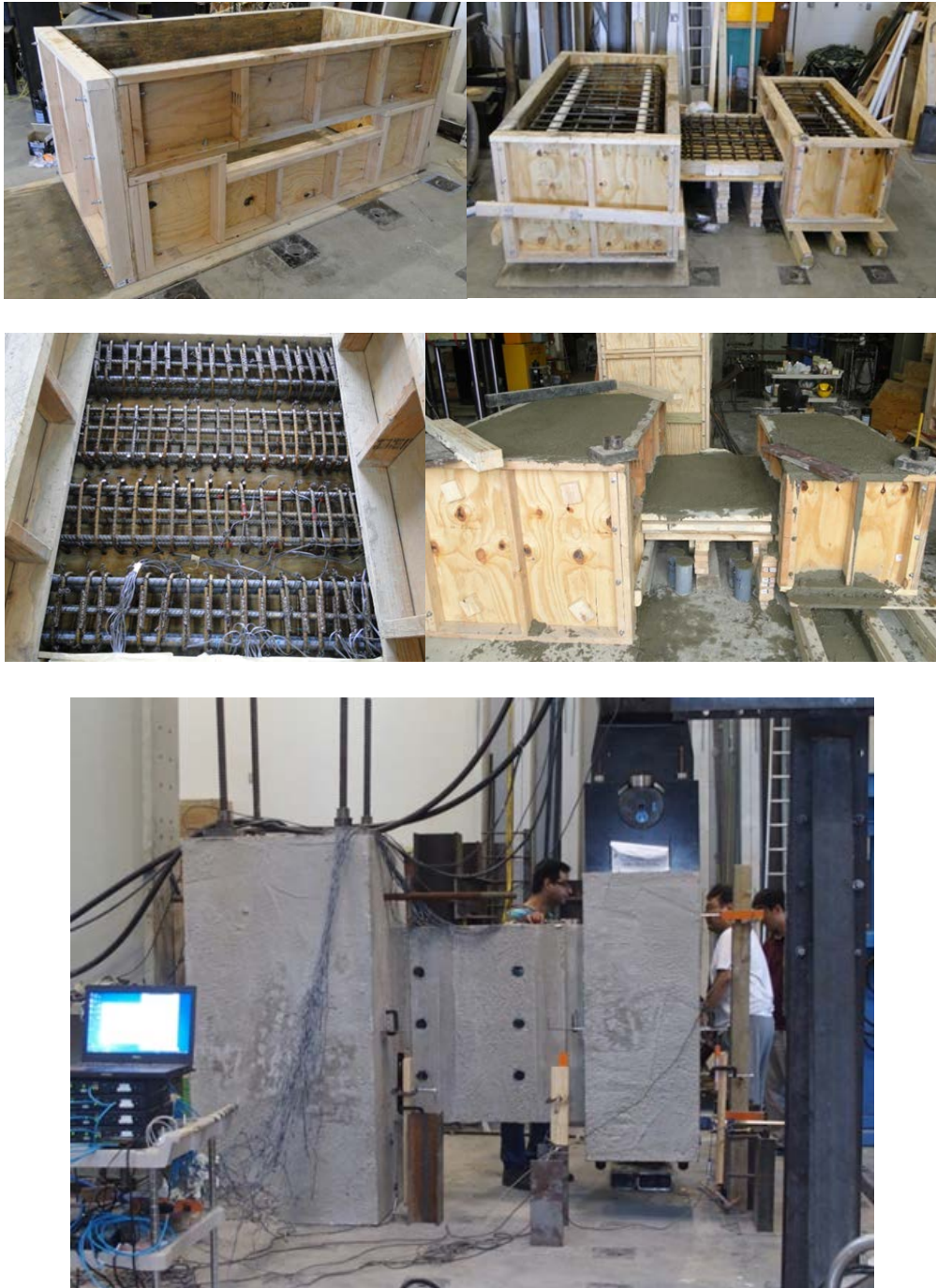
Figure 3-10 Construction of the Squat wall
