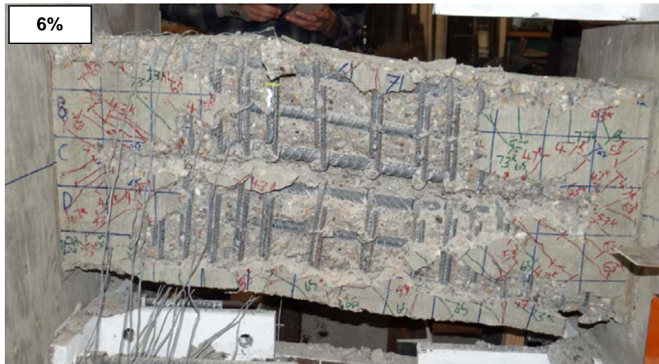
Figure 4.17 Crack pattern and damage progress of DBCBs with 1" gap width
