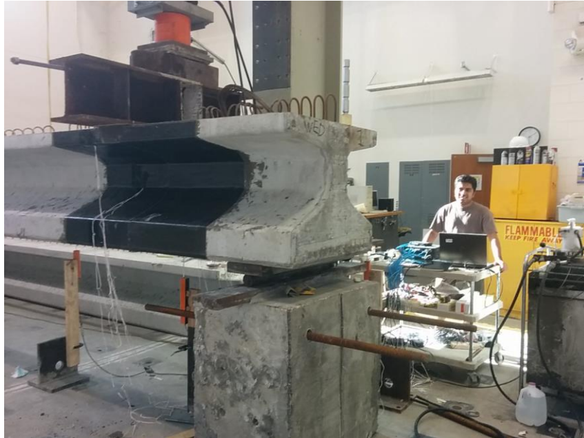
Figure 6-19 – Loading setup for shear test GS1
