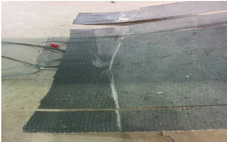
Figure 6-18 - FRP debonding at maximum loading GF2
