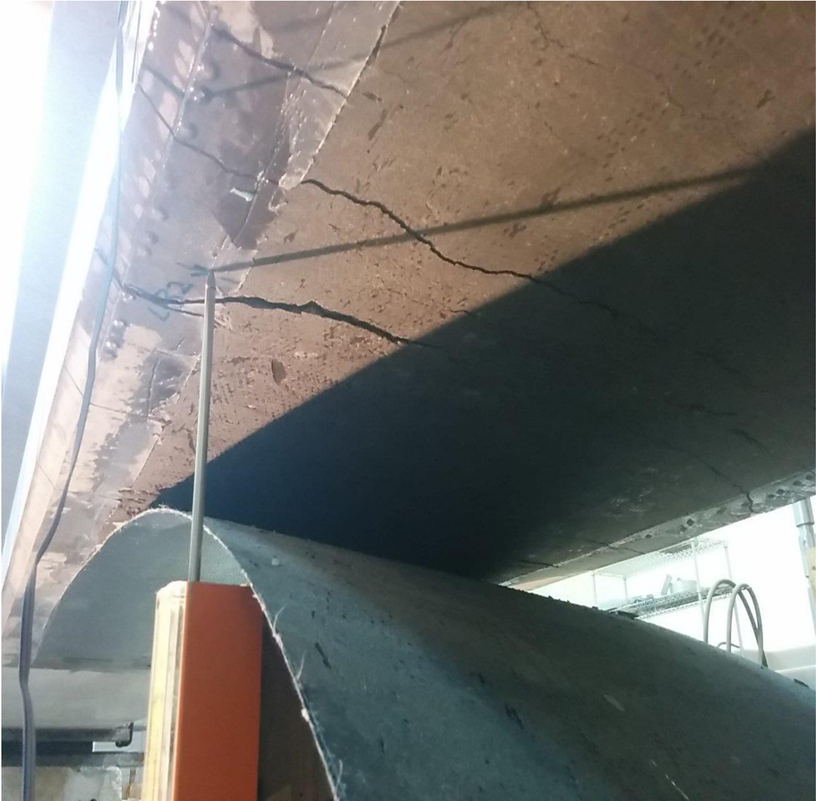
Figure 6-16 - FRP debonding at maximum loading GF2
