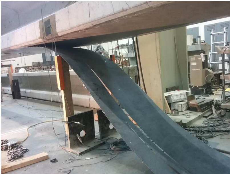
Figure 6-14 - FRP debonding at maximum loading GF2
