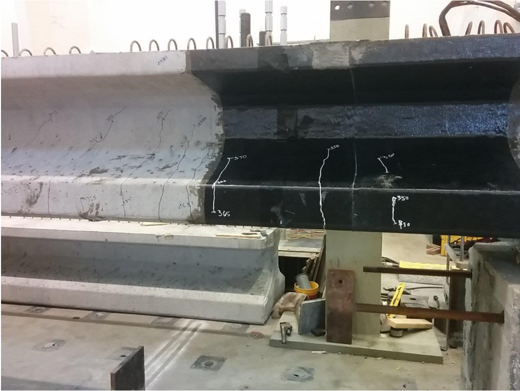
Figure 6-21 – Observed cracks due to loading GS1
