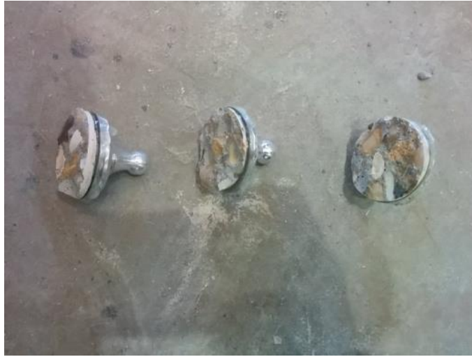
Figure 4-12 – Samples from the Pull off test
