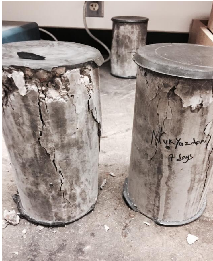
Figure 4-2 Specimens after strength test
