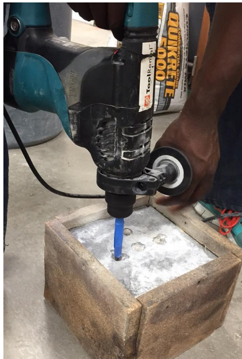
Figure 5-8 Collecting powdered samples using rotary hammer
