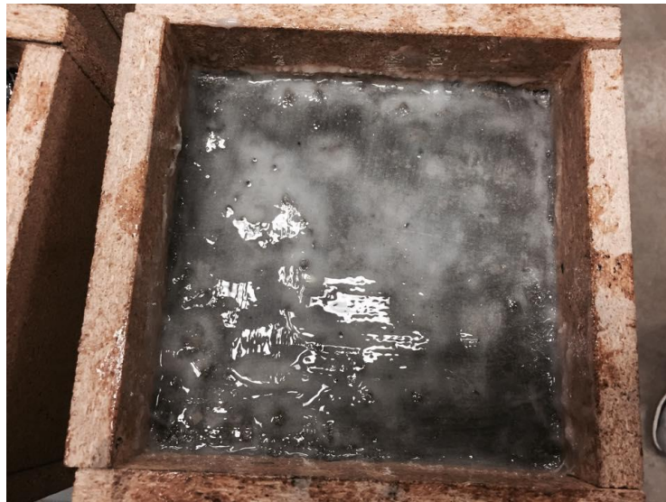
Figure 5-5 Tyfo WEB composite installed on concrete specimen
