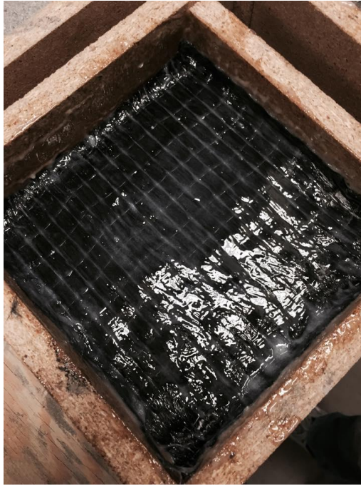
Figure 5-4 Tyfo SCH-41 composite installed on concrete specimen
