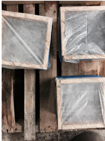
Figure 5-7 Concrete specimen being taped with polythene sheet
