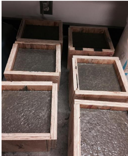
Figure 5-2 Concrete specimens before FRP and epoxy installation
