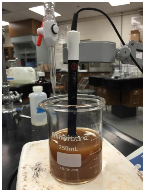
Figure 5-13 Silver/Sulfur Electrode being submerged in to beaker
