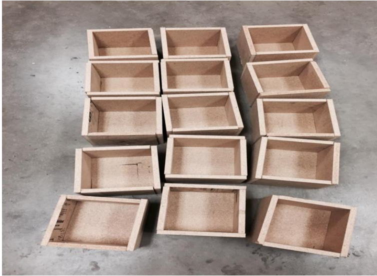
Figure 5-1 Plywood molds for casting concrete
