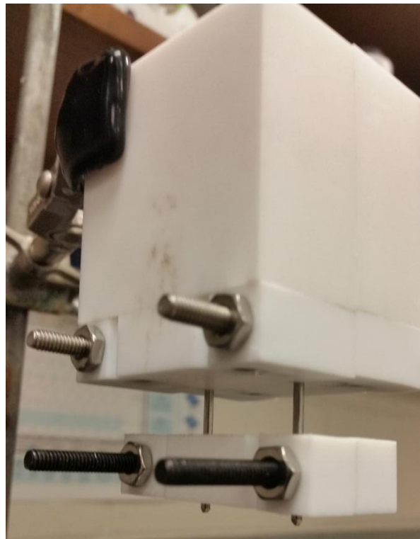
Figure 6-4 Photo of the spacer at the probe end
