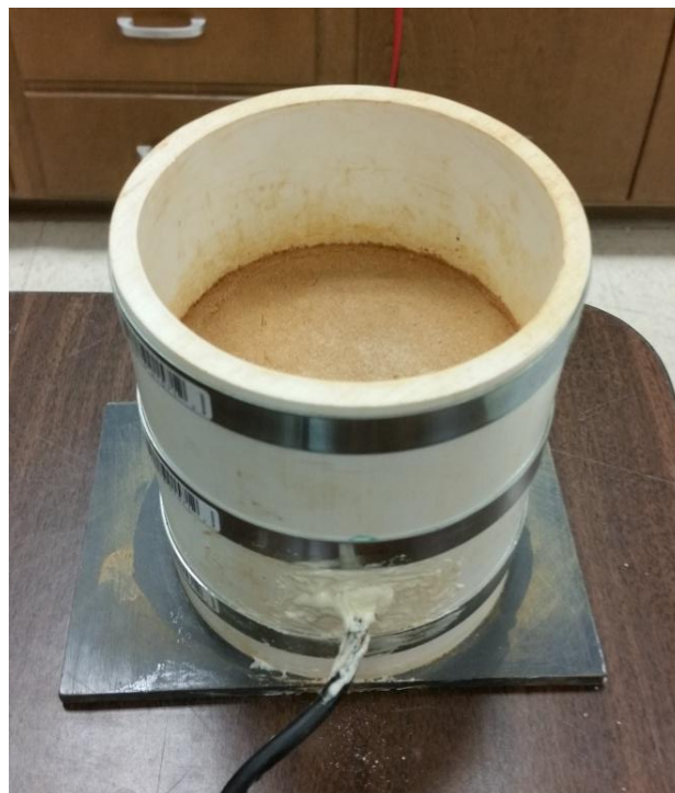
Figure 6-19 Photo of test silty sand in desorption test
